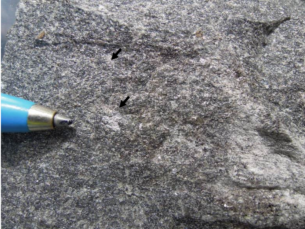
Silvery arsenopyrite and löllingite in fine-grained metasandstone.
