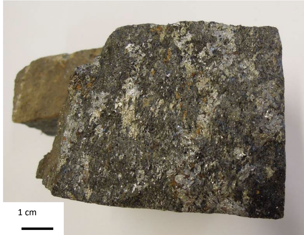
Discrete shear zone in a metasedimentary rock with silvery arsenopyrite and löllingite. Yellowish metallic minerals are pyrite and pyrrhotite.
