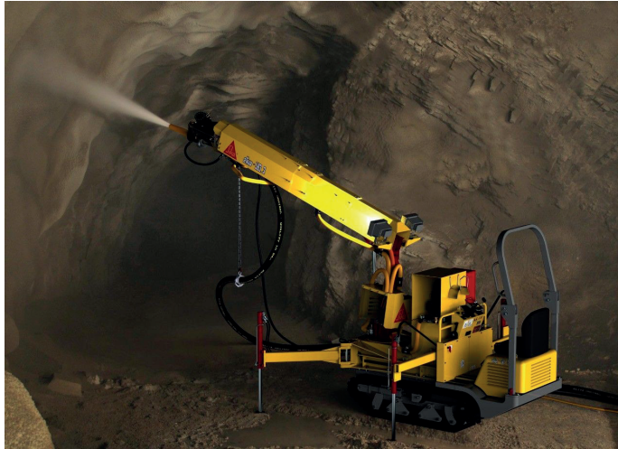
Figure 1.1: Spraying of shotcrete with a remotely controlled machine. Photo from Sika.
