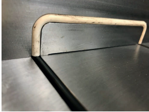
Figure 35. The junction of O-ring for sealing side of aperture plate and O-ring for sealing bottom plate. The good seal between both O-rings after tightening plates is important for successful water test.
