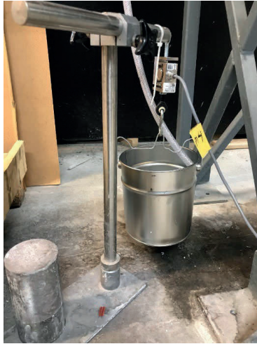
Figure 33. Mass sensor with bucket for grout flow recording.
