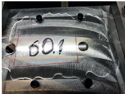
Figure 7. Example of detected leakage in aperture plate.
