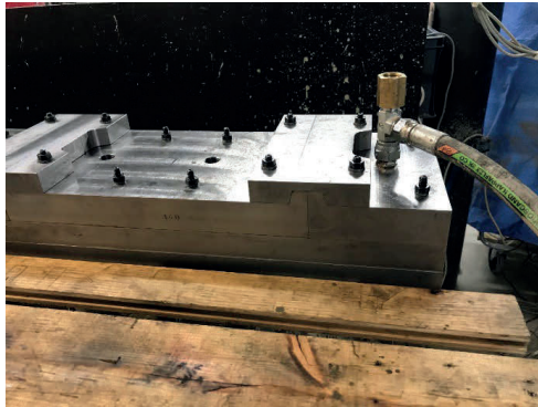
Figure 36. Upgraded position of the grout inlet hose. The top entrance of “T” connection is used for installation pressure sensor.
