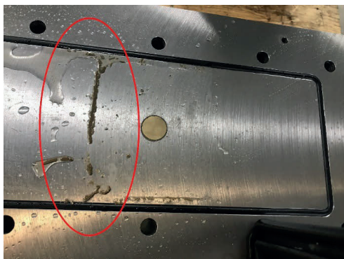
Figure 39. Water failed to reach outlet plate due to plug at the inlet plate. The plug was formed of hardened grout particles carried by water from not clean enough distribution unit walls.
