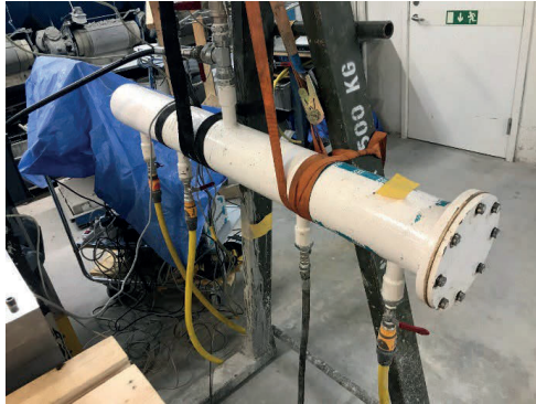
Figure 37. Distribution unit which is filled with grout before testing and pressurized with nitrogen.
