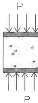
Figur 3.2.2 Tryckhållfasthetsprov The compressive strength test set-up
