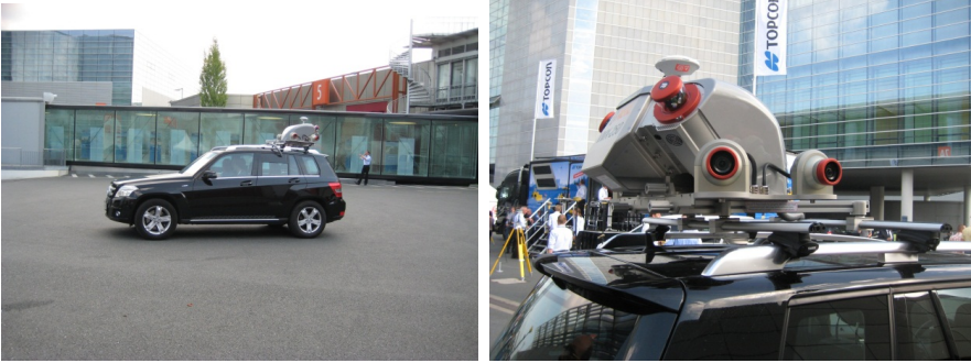
Figure 2-7. Topcon mobile scanning system ( www.topcon.com ).
