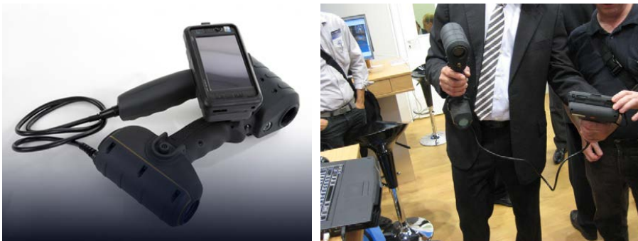
Figure 2-10. Hand-held scanner of Mantis Vision.
