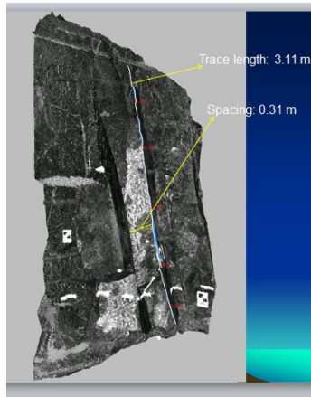
Figure 5-7. Measuring fracture length and spacing in 3D scanning point clouds.
