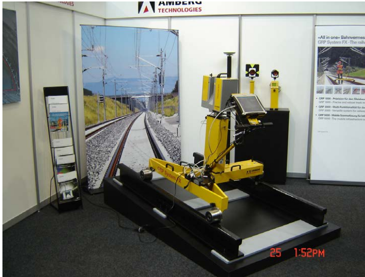
Figure 2-5. Amberg GRP scanning system developed for railway scanning [27].
