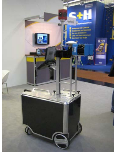
Figure 2-9. S+H trolley mobile scanning system ( www.intergeo.com ).
