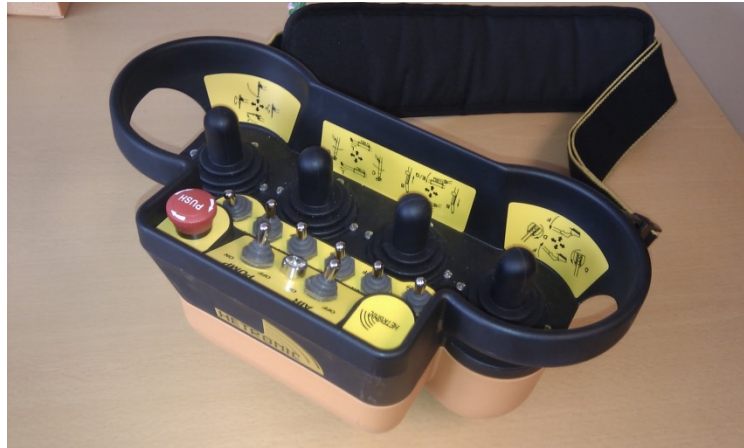
Figure 5: Example of a control used by shotcrete operators.
