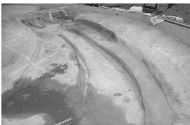
Figure 4. The design of the spillway that gave the most favorable flow pattern in the physical model tests.
