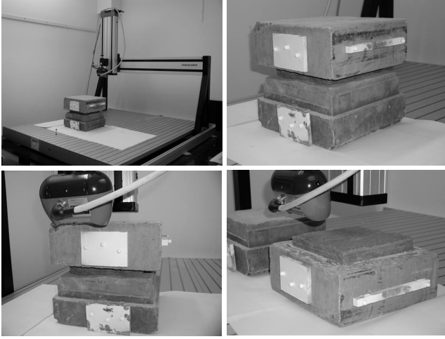
Figure 2. 3D-laser measuring of the concrete replica at the Laboratory.
