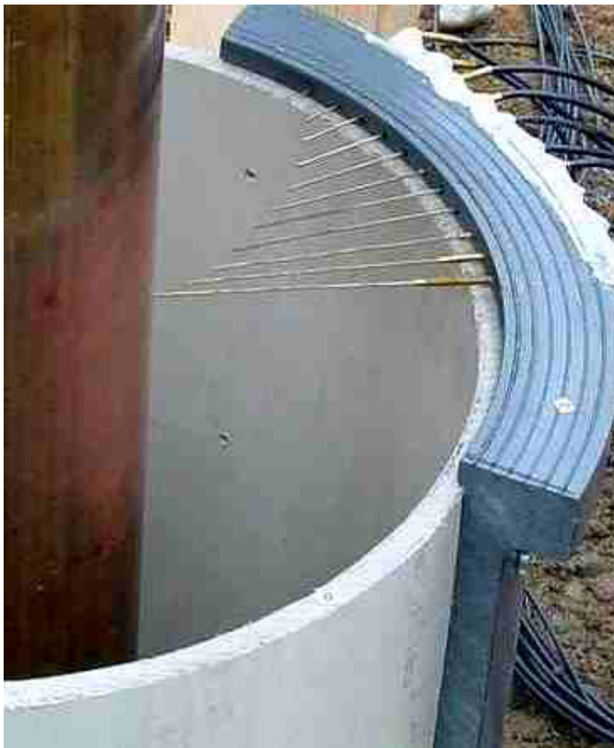
Figure 2. Photo of the mounted contact pins with gauge jig.
