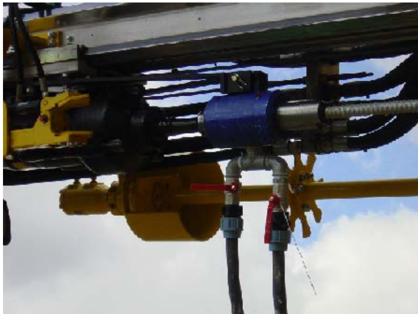
Fig.7: Rotary Injection Adapter with dual Flush inlet
