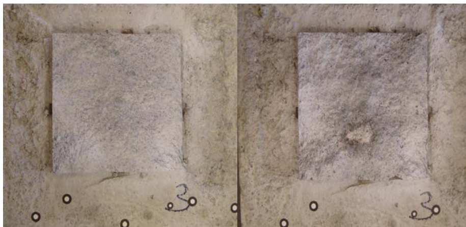
Figure 3.2 Sample 3 before (left) and after (right) shearing.
