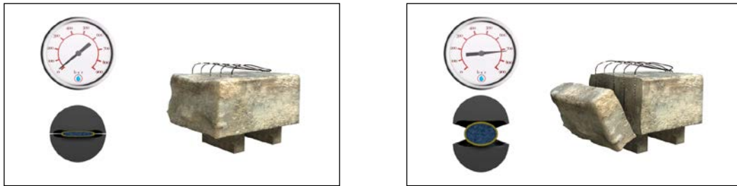
Figure 3 Installed rock splitters before (left) and after (right) pressurization
