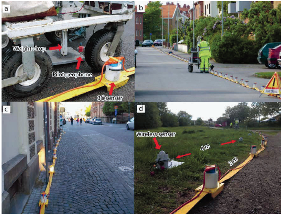
Figure 2. Field photos showing (a) seismic source (a 110-kg accelerated weight drop) used in this study to generate seismic signal and a close-up of a 3C sensor mounted on the sled, (b-c) example field and ground conditions in the city of Varberg and (d) combined wireless and streamer sensors (see lines 2 and 3 in Fig. 3).
