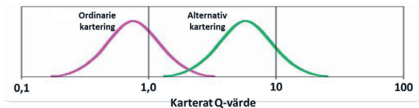
Figur 7: Jämförelse mellan olika utförares kartering av samma tunneldelar på projekt Ådalsbanan. Comparison between rock quality classifications executed in identical tunnel parts by different organizations in the Ådalsbanan project.
