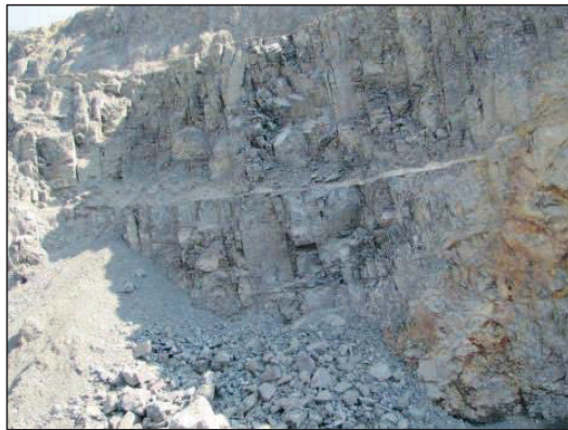
Figure 11: Calcite/Talc layer interpreted as following the base of the VRM (Consolidated) Basal Failure on Clay Layers
