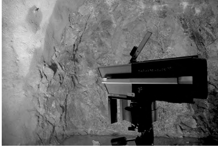
Figure 9. Photograph of the JointMetriX3D image scanner on site.
