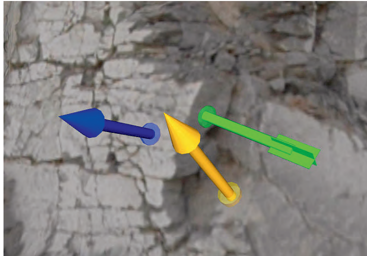
Figure 3. Individual orientations directly measured in a 3D image. The arrow is the normal vector of the orientation indicating an overhang (tail) or a non-overhang (spike).
