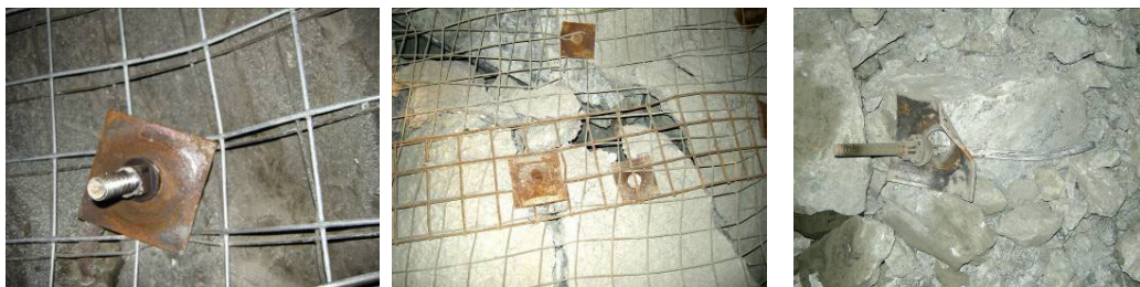
Figure 5 Examples of the various and frequently occurring support failures: Left – bent and twisted Rebar stripped of rock fragments; Centre – SplitSet head failure/lost connection to liner; Right – Swellex sheared off. Elsewhere the domed plate and spherically-seated nut performed comparatively well (Below, Left). Ultimately the failed rock & shotcrete was only held together by surviving cone bolts and screen straps (Below, Centre), the shotcrete acting like large rock bolt plates. A number of Modified Cone Bolts were observed to have failed in tension, as evidenced by “necking” (Below).
