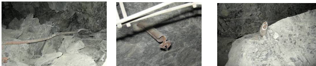
Figure 5 Examples of the various and frequently occurring support failures: Left – bent and twisted Rebar stripped of rock fragments; Centre – SplitSet head failure/lost connection to liner; Right – Swellex sheared off. Elsewhere the domed plate and spherically-seated nut performed comparatively well (Below, Left). Ultimately the failed rock & shotcrete was only held together by surviving cone bolts and screen straps (Below, Centre), the shotcrete acting like large rock bolt plates. A number of Modified Cone Bolts were observed to have failed in tension, as evidenced by “necking” (Below).
