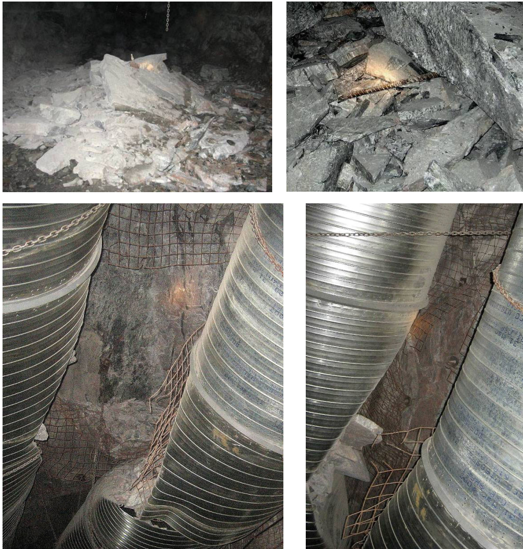
Figure 1 Rockburst/ground support failure in a mine ramp. Upper Left: 11 tonnes of rock fall-out debris; Upper Right: Single sheared \frac{3}{4} -inch Rebar; Above Right/Left: Site of bolt and mesh failure in back of ramp.
