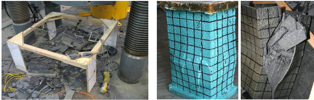
Figure 11 Post-test appearance of failed sample given 3 different liners: Fibre-Reinforced Shotcrete (Left), 3M TSL-Version 1 (Centre) and Rockweb (Right). The stiff, brittle shotcrete demonstrated minimal capacity to manage the sample's violent post-failure response, while the thin, deformable 3M liner, though tearing locally, demonstrated the superior capacity of the 3 tested.
