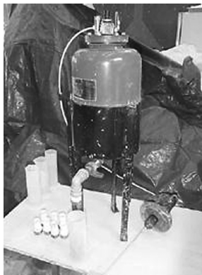
Figure 9 Penetrability meter developed by Eriksson and Stille (2003)
