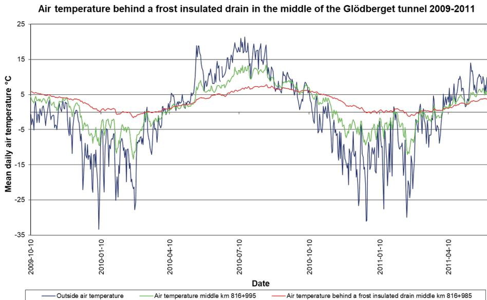
Figure 4.7 Temperature behind a frost insulated drain mat, Glödborget 2009-2011 (Andrén et al., 2022).
