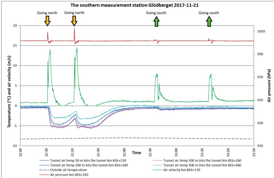
Figure 4.3 Four train passages through the Glödsberget tunnel, the southern measurement station (Andrén et al., 2022).
