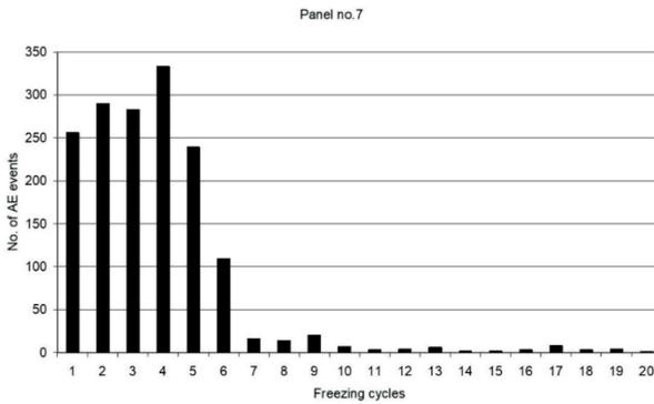
Figure 5.5 Number of AE events for each freezing cycle for panel number 7 with access to water during freezing (Andrén et al., 2020a).
