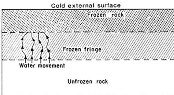
Figure 2.11 Frozen fringe – the zone between the frozen and the unfrozen layers (modified from Walder and Hallet, 1985).
