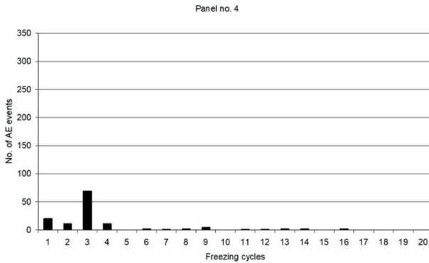
Figure 5.6 Number of AE events for each freezing cycle for panel number 4 without access to water during freezing (Andrén et al., 2020a).
