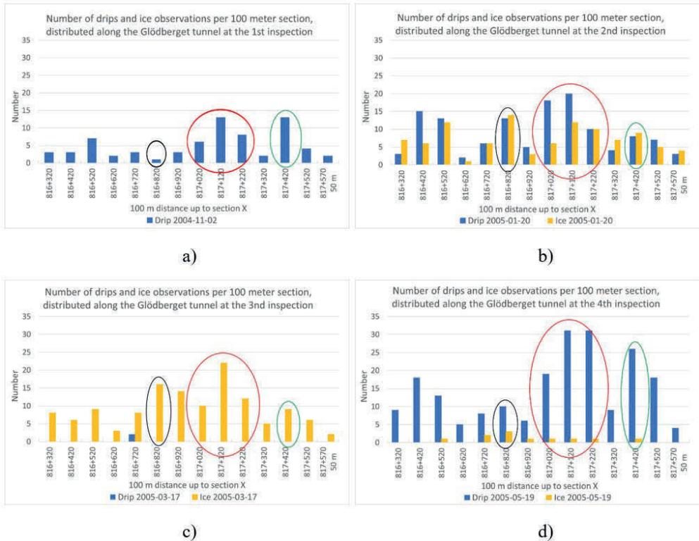
Figure 3.3 Number of drips and ice observations per 100 m section for the Glödborget tunnel, 2004/2005 (Andrén et al., 2023).
