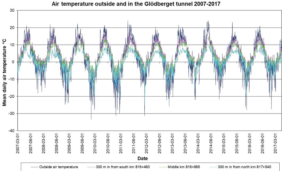
Figure 4.13 Daily mean air temperatures outside and in the Glödsberget tunnel 2006-2017.
