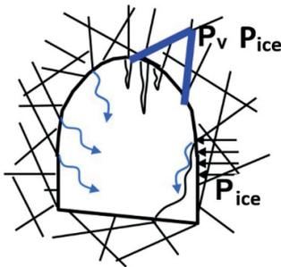
Figure 2.1. Ice loads ( $P_{ice}$ ) arising when leakage occurs in the frost zone (Andrén, 2004).
