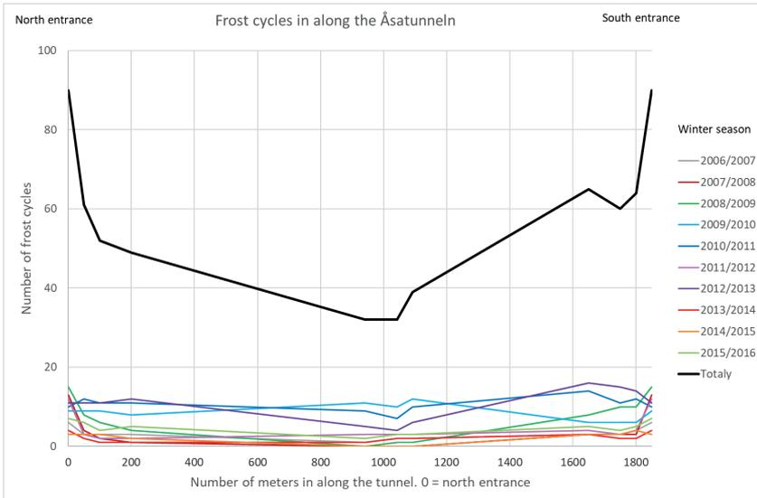
Figure 4.9 Number of frost cycles along the Åsa tunnel.
