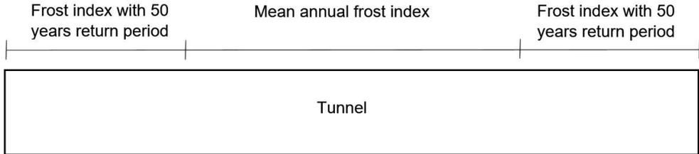
Figure 2.7 Current requirements for the frost index at different sections inside a tunnel.
