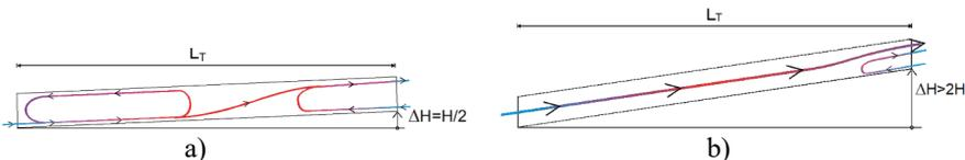
Figure 2.10 a) Class II Case C  $\Delta H = H/2$  No air flows out of the tunnel at the lower entrance.
