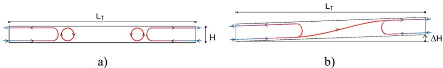
Figure 2.9 a) Class I Case A  $\Delta H = 0$  Two convection loops with no contact with each other.
