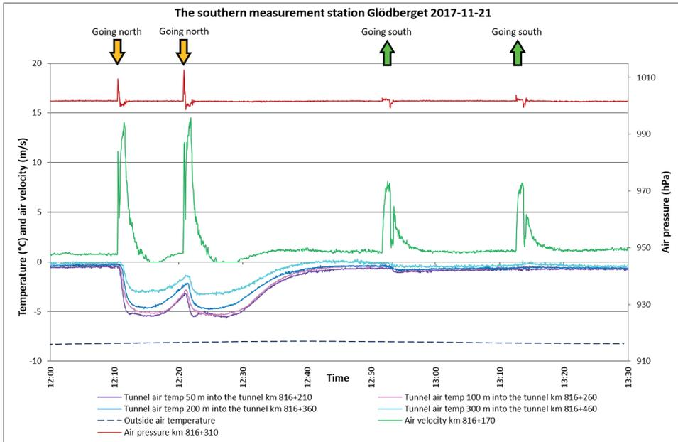
Figure 4.4 Four train passages through the Glödsberget tunnel, the southern measurement station (Andrén et al., 2022).
