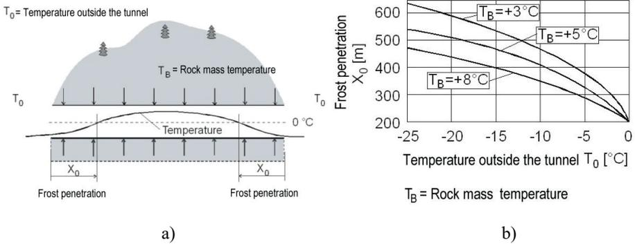
Figure 2.8 Frost penetration (figures modified from Sandberg et al., 2002).
