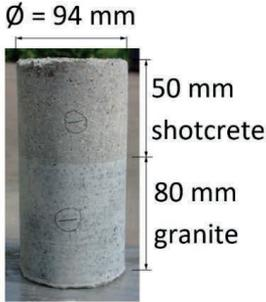
Figure 5.7 Test sample of shotcrete-rock core (Andrén et al., 2020a).
