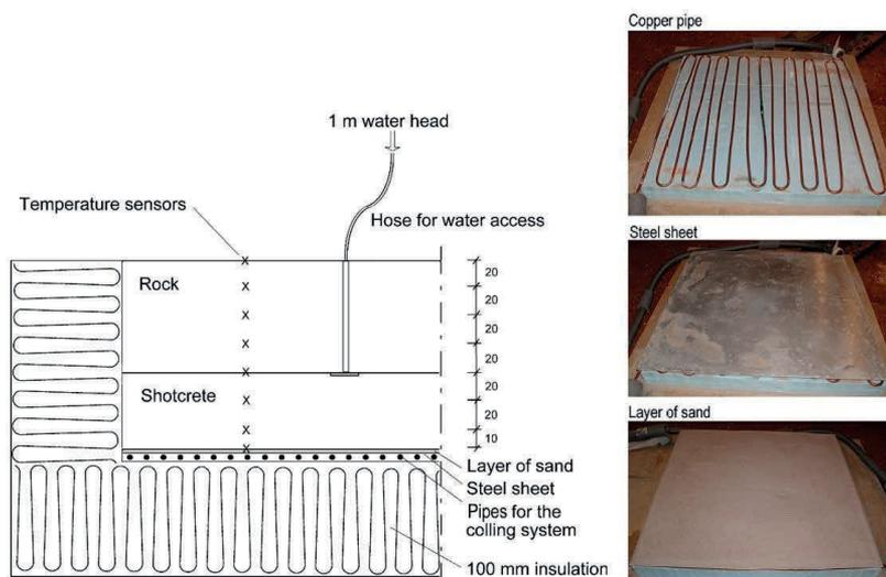
Figure 5.3 Arrangement of the freeze-thaw test experiment (Andrén et al., 2020a).
