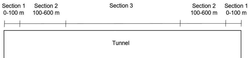
Figure 4.11 Future division of tunnel sections for different frost indexes inside a tunnel.
