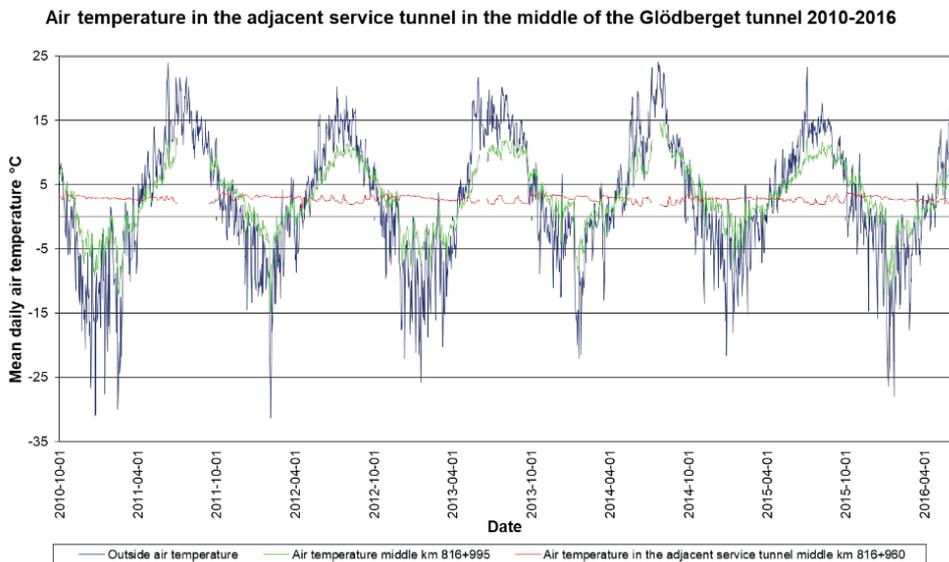
Figure 4.6 Temperature in the adjacent service tunnel (red curve), in comparison to outside temperature (blue) and middle section tunnel air temperature (green), Glödsberget 2010-2016.
