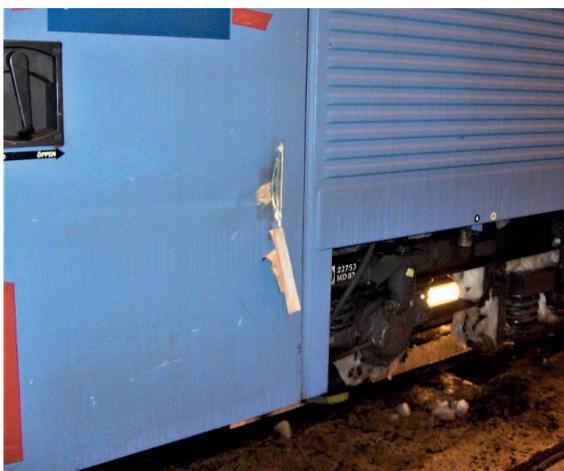
Figure 3.15 Sheet metal damage (Photo: Veolia transport).
