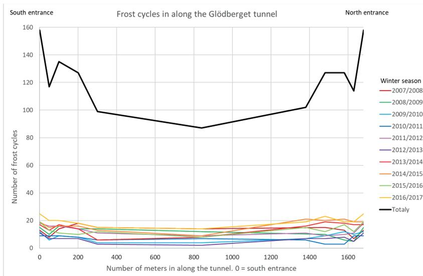
Figure 4.8 Number of frost cycles along the Glödberget tunnel.
