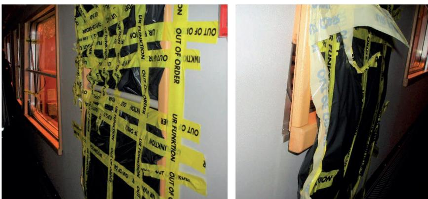
Figure 3.16 Deformed window frames (Photo: Veolia transport).
