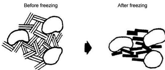
Figure 2.2 Restructuring of clay particles when freezing (after Chamberlain and Gow, 1978 – from Johansson, 2005).
