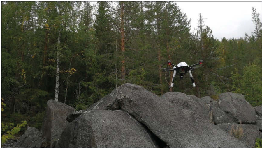
Figure 9. An Explorian (XLT) Pitchup drone, mounted with a Sony Alpha high-resolution camera taking off to perform photogrammetry.
