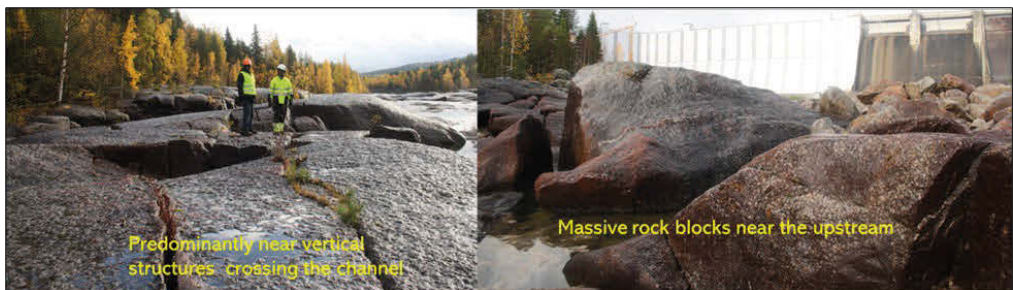
Figure 29. Widely spaced vertical structures that form massive rock blocks.
