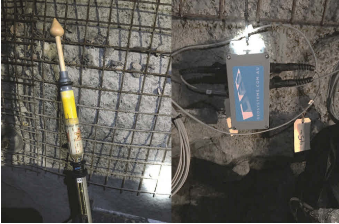
Figure 13: Fully prepared HID-Cell (left) and Yieldpoint D4Logger (right).
