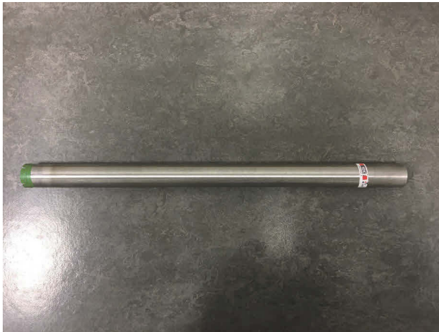
Figure 14: 1-m long diamond core barrel adapted for use with cable bolter.
