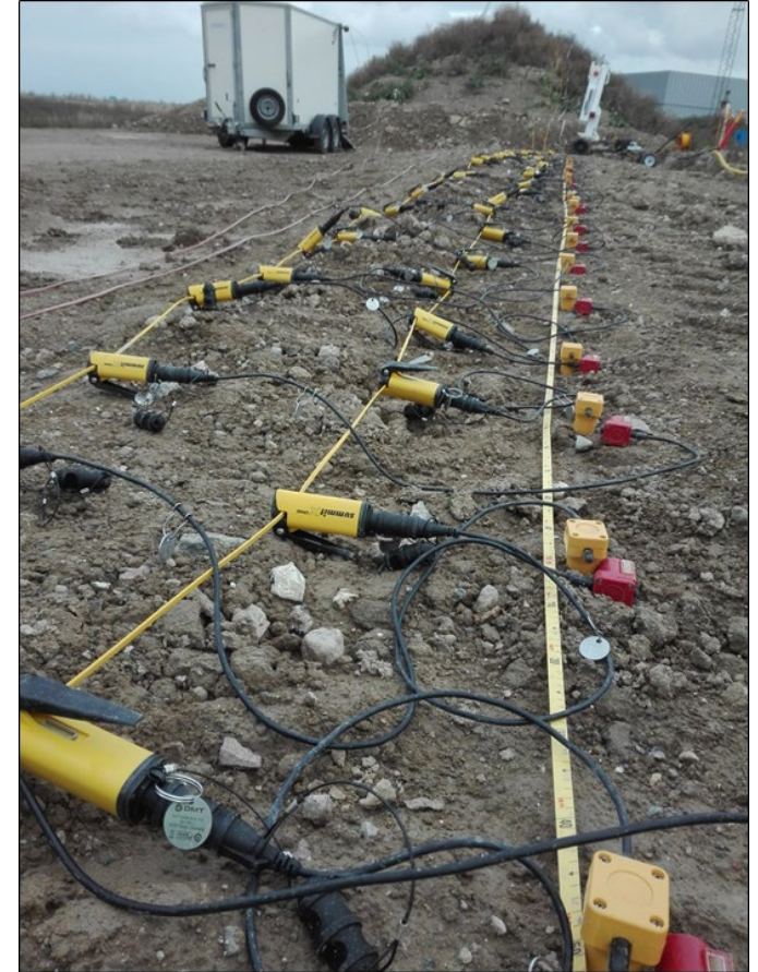
Example of geophones layout with 0.5 m spacing and 4.5 Hz geophones. Yellow receivers are the vertical component geophones, while the red ones are the horizontal (in-line) component geophones.
