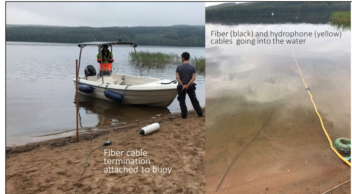
Workboat and placement of the seismic cables close to shoreline.
