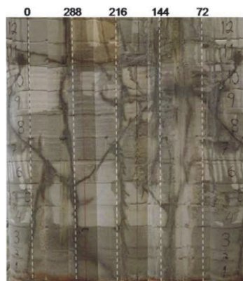
Figure 49. After (Fransson et al., 2017), lower part of bentonite parcels from KO0018G01 with wetting marks after their extraction. Bentonite blocks 1 to 12 identified on the right hand side of the illustration,
