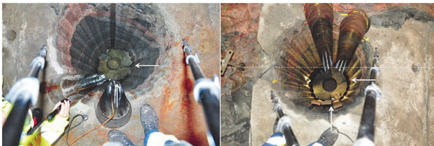
Figure 50. Boreholes after dismantling. KO0017G01 on the left and KO0018G01 on the right. The additional fractures are marked in white arrows.
