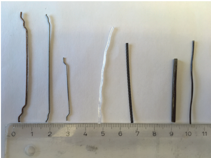
Figure 2.6: Different type of macro (structural) fibres. From left to right, steel fibres with various end-hooks (1-3), synthetic fibres (4-5) and basalt fibres (6-7).
