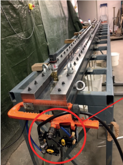
1. Ball-valves, 2. Pneumatic actuators, 3. Solenoid valve, 4. Asymmetrical recycler timer
