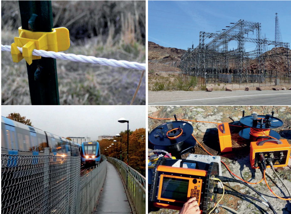
Figure 8. Different types of known sources that affect the measured potential and their typical signal characteristics: electrical fence – spikes (top left), power grid – harmonic noise (top right), tram running on DC – anthropogenic background drift (bottom left), DCIP instrument – square pulse train (bottom right).
