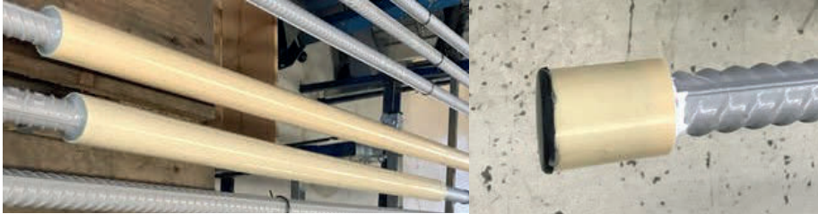
Figure 3-2. Preparation of defects and end plug (to the right) on ordinary rebar bolts.
