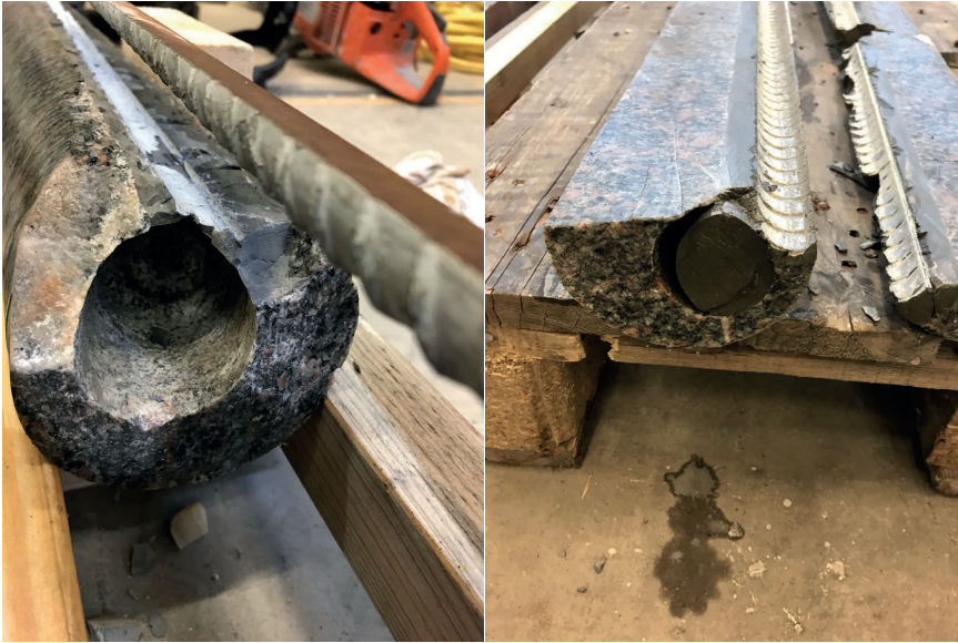
Figure 3-14. Core from bolt the TASJ7 – a cavity present at the length 2.3 m (left), and a partly filled bolt hole on the opposing core piece (right).
