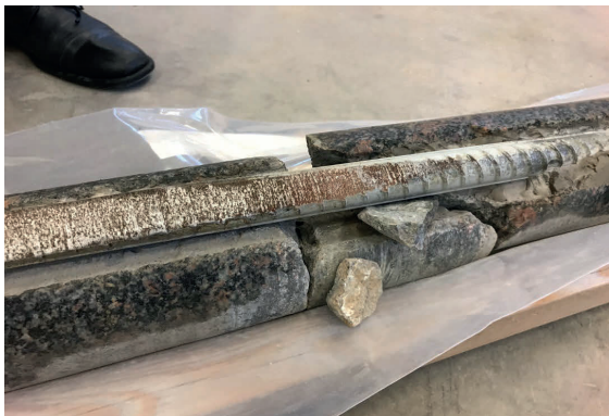
Figure 3-16. Core from the bolt TASJ11– natural fractures and part of the bolt without grout at 0.5-0.7 m bolt's length.
