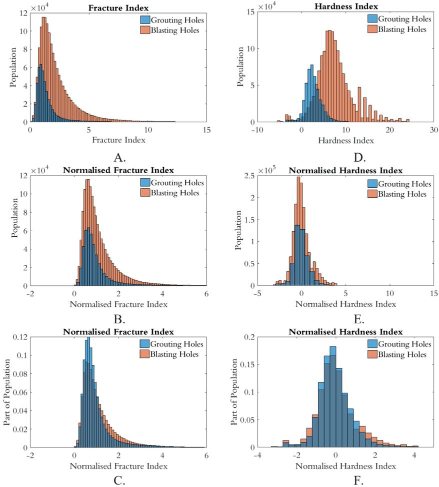
Figure 5.21 Normalisation procedures for Fracture Index and Hardness Index for MWD data for Tunnel 213 and Tunnel 214 at Stockholm bypass. The raw Fracture Index (A) and the normalised data (B) show a similar distribution for the grouting and blasting hole Fracture Index (C). The raw Hardness Index (D) shows a normal distribution (E); the distribution is similar for grouting and blasting (F).
