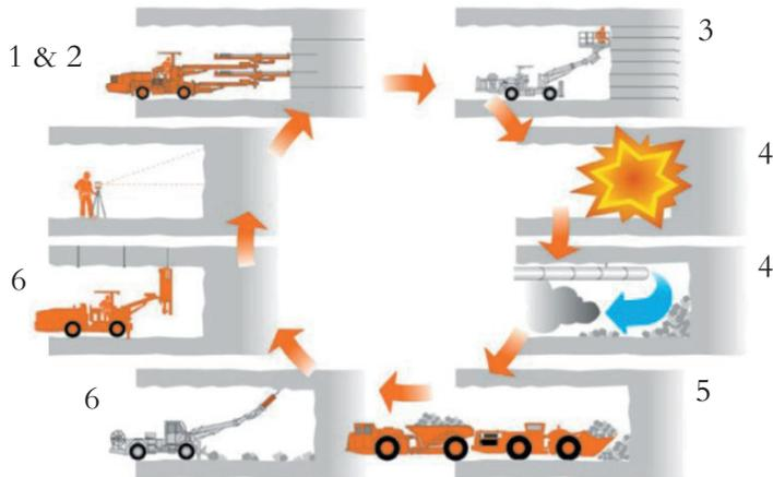
Figure 3.1 Excavation cycle in tunnel excavation (Modified after Tamrock, 1999).
