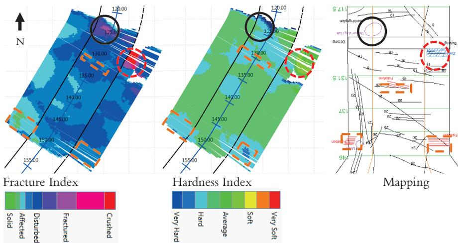
Figure 5.26 Fracture and Hardness Indices based on the grout holes, and mapping of the access tunnel; the encircled areas indicate fractured areas and the rectangles show the effects of the foliation.
