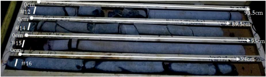
Figure 5.13 Cores #12, #14, #15 and #16 from TAS04 tunnel. The cores show a more extensive fracturing at the start of the drill hole, these fractures were determined to be blast induced.
