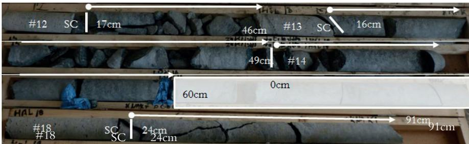
Figure 5.11 Cores from Hole #12, #Hole #13, Hole #14 and Hole #18 of Tunnel 214. The cores show a more extensive fracturing at the start of the drill hole, the majority of the fractures were newly formed (SC = Sprayed Concrete).
