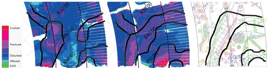
Figure 5.24 Fracture Index for section 848 to section 820 (28m) in Tunnel 214 showing grout holes on the left, blast holes in the middle and mapping on the right. The black lines indicate the shape and orientation of the fracture zones in the MWD data and tunnel mapping.
