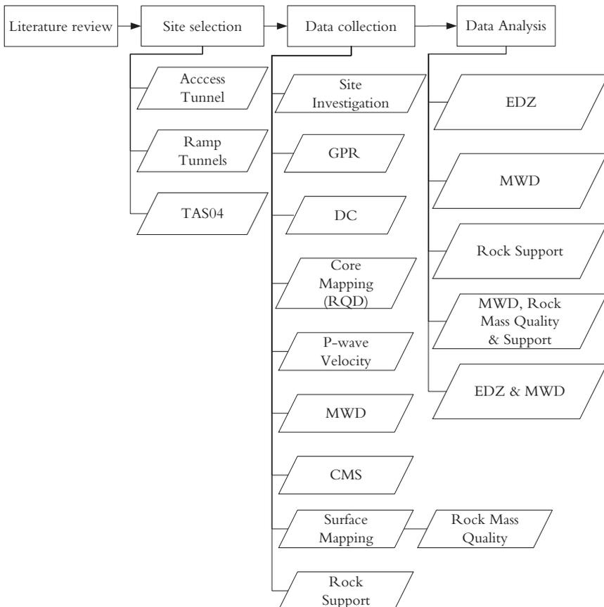
Figure 2.1 Methodology to study excavation damage in tunnelling.
