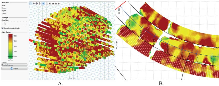
Figure 2.5 Penetration rate of one blast round in Underground Manager of section 796 in Tunnel 214 (A) and the interpolated penetration rate on the tunnel contour in the first 65 m of Tunnel 214 (B).
