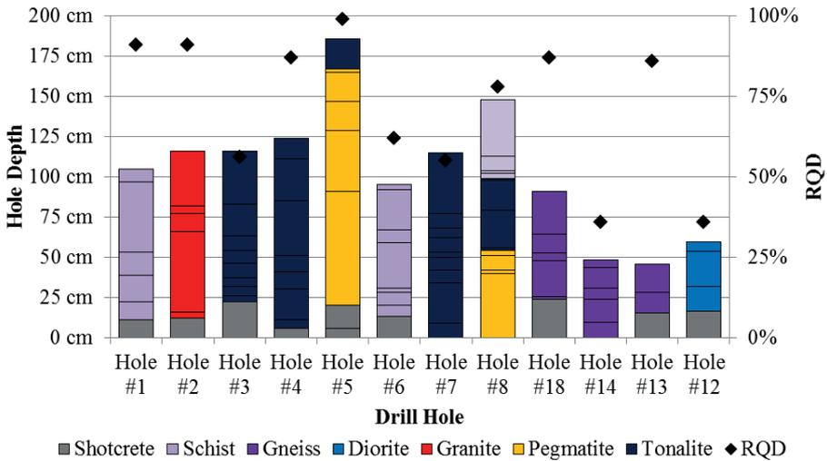
Figure 5.9 Drill core mapping from tunnel 214 and the Veidekke access tunnel for the blast damage investigation. The left axis displays the total core length; the black lines within the core display the separation of the core parts. The black diamonds in the figure show the RQD with their values on the right axis. The RQD values ranges from 30% to 100%. This value is a combination of natural and blast induced fractures.
