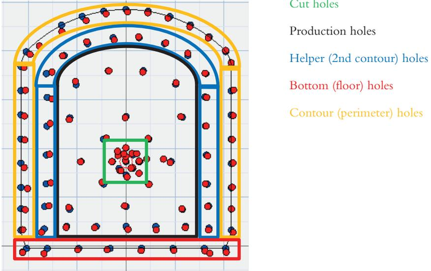
Figure A.1 Schematic layout of a blast hole drilling round for a tunnel blast. The blue dots show the drill plan and the red dots the drilling performance.
