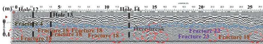
Figure 5.4 Ground Penetrating Radar showing recorded fractures (red circles) for left wall section 848, the tunnel portal, to section 827, 21m into the tunnel, in Tunnel 214 at the Stockholm bypass; the majority were related to fractured mapped, and others are likely to be caused by blasting. The blue line shows the zone of dispersion (micro fracture reflections) in the rock mass.
