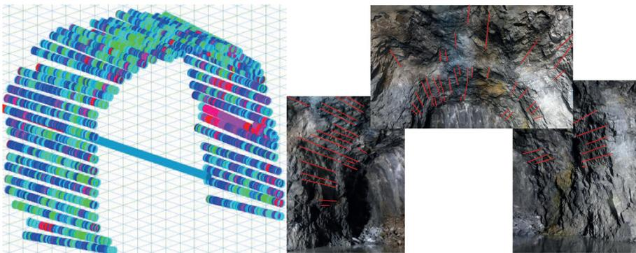
Figure 5.1 Blast holes and Half Casts in a section in Tunnel 213 (photographs modified after ÅF 2016).
