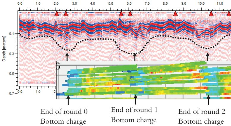
Figure 5.5 GPR and drilling data for the left wall of TAS04 tunnel showing an increase of the extent of the GPR blast damage at the drill hole bottoms with a higher charge concentration. The red triangles are marking points manual added during the recording and have no influence on the recorded data. The black dashed line is the interpretation of the extent of the blast damage zone.
