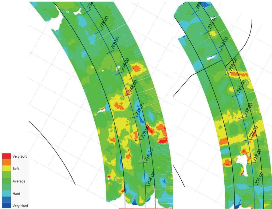
Figure 5.23 Hardness Index for section 200 to section 290 (90m) in Tunnel 213 showing grout holes on the left and blast holes on the right. Softer rock is massed in section 218 to section 243 (25m).
