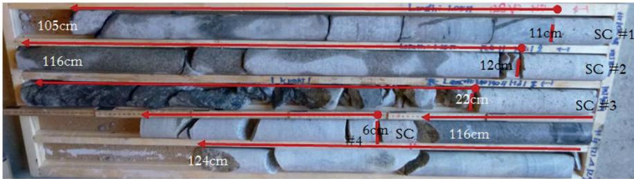
Figure 5.10 Cores from Hole #1 to Hole #4 from the Veidekke access tunnel. The cores are more extensively fractured at the start of the drill hole, most of the fractures were newly formed (SC = Sprayed Concrete).
