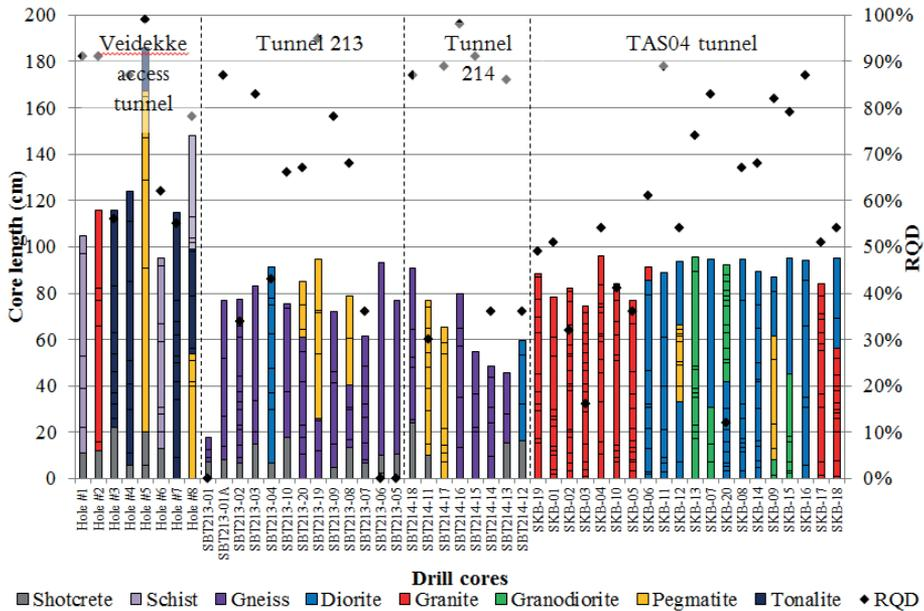
Figure 5.12 Drill core mapping the four investigated tunnels. The left axis displays the total core length; the black lines within the core display the separation of the core parts. The black diamonds in the figure show the RQD with their values on the right axis. The RQD values range from 0% to 100%. This value is a combination of natural and blast induced fractures.
