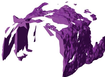
Figure 5.2 Over-break based on the drill log in Tunnel 214, from sections 845 (3m from tunnel entrance) to 831 (14m from tunnel entrance) and the volumetric scan (CMS).
