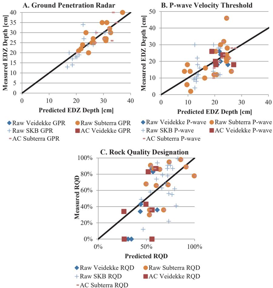
Figure 5.28 Correlation of the measured and predicted (by the factors derived from MLR analysis) extent of the blast damage at the three sites based on the GPR (A), P-wave velocity (B) and RQD (C).
