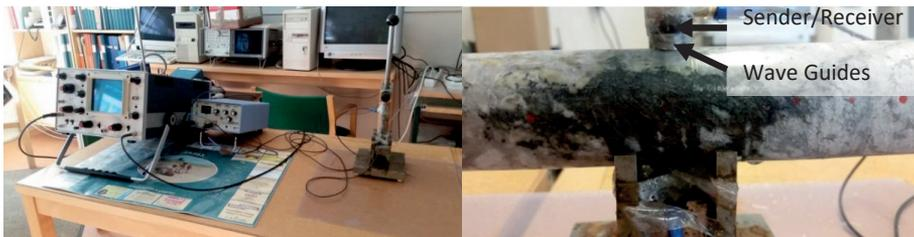
Figure 2.3 Setup for diametrical P-wave measurements on the collected drill cores.
