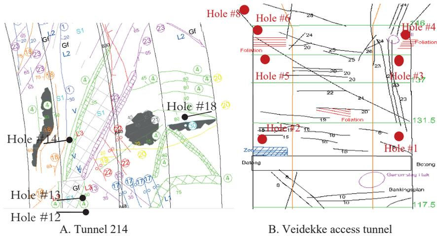
Figure 5.8 Fracture mapping and diamond core hole locations of Tunnel 214 (A) from the tunnel entrance (section 848) to 21m into the tunnel (section 827) and the drill cores taken in the Veidekke access tunnel (B) from section 117.5, 67.5m into the tunnel to the entrance to gallery at section 146, 96m into the tunnel.
