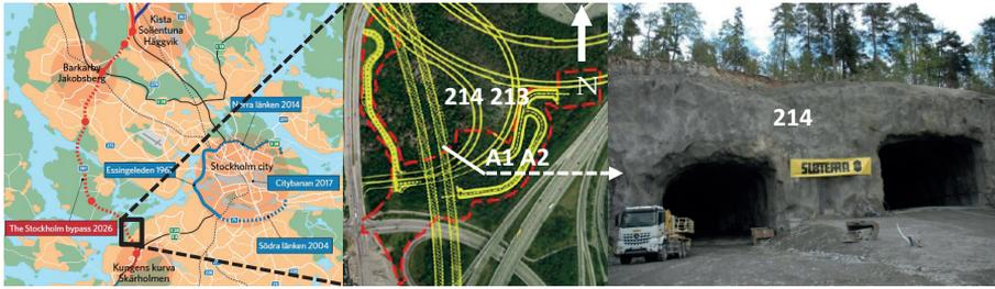
Figure 4.2 Stockholm bypass and Tunnels 213 and 214 location, layout and tunnel entrances (Illustrations courtesy of Trafikverket).
