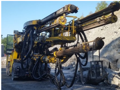
Drill rig for data collection
