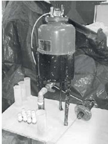
Fig. 6 Penetrability meter developed by Eriksson and Stille (2003)
