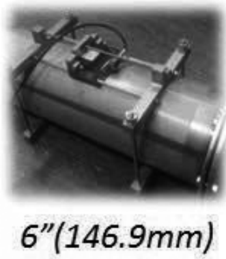
Figure 18. Incipientus ILR in-line rheometer 6" non-invasive ultrasound transducer
