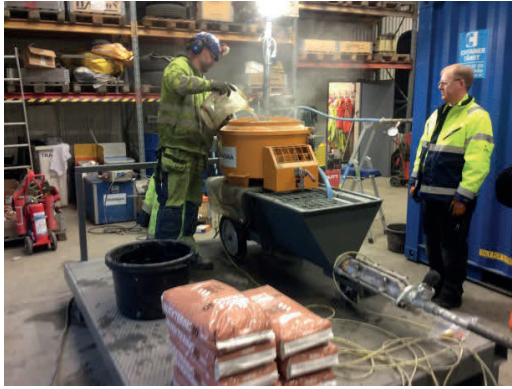
Figure 26. Portable commercial grouting pump and mixer for field use.
