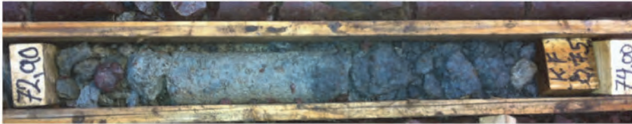
Figure 7. Fault gouge in core 13VEC10K. OBS the upper photo is of fault gouge at about 76 m and the lower is at about core length 72,9 m.
