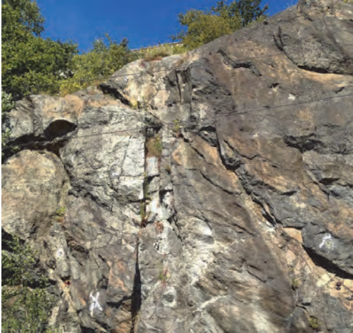
Figure 24. An example of a rock wall from Lidingö where the relative movement were exposed as normal faulting of pre-existing fractures (site Lidingö (07) surface no. 002) indicated as 07-002 in Table 1.
