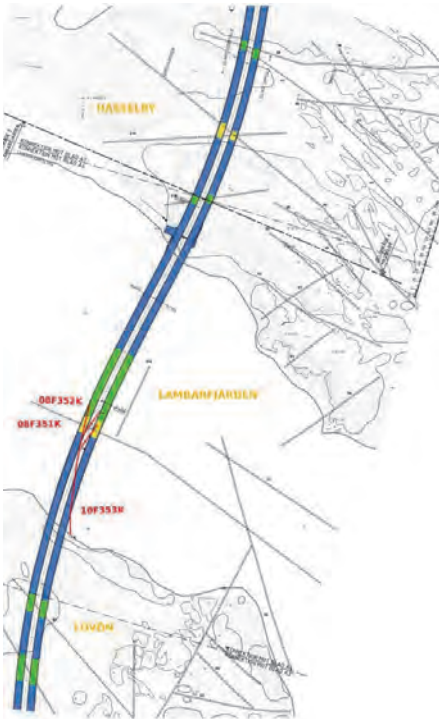
Figure 5. Results from the investigation by Vass, 2012. The coloured lines are the tunnels for the project Förbifarten, where the colours denotes the expected rock quality. The bore holes are indicated in red.
