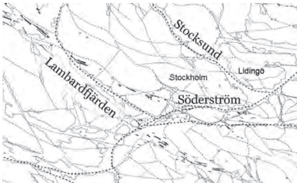
Figure 4. Part of map of fault and fracture zones in the Stockholm area from Stålhös (1969) with the fault names along the structures. The thick black lines are dolerite dykes (indicating possible extensional phase) crossing the area, the thin dashed lines are fracture zones according to Stålhös (1969).
