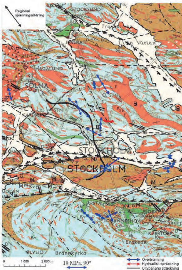
Figure 15. Geology and structures as well as direction and average value for the maximum horizontal stress axis for in-situ stresses in the Stockholm area. The regional stress direction is presented in the upper left corner. The figure is a combination of several maps and is thus an estimate. From Perman & Sjöberg, 2007, the geological map is from Stålhös (1969).
