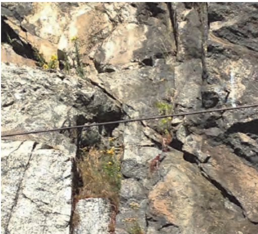
Figure 25. An example of normal faulting of pre-existing fractures from Lidingö (07) surface no. 002, indicated as 07-002 in Table 1.
