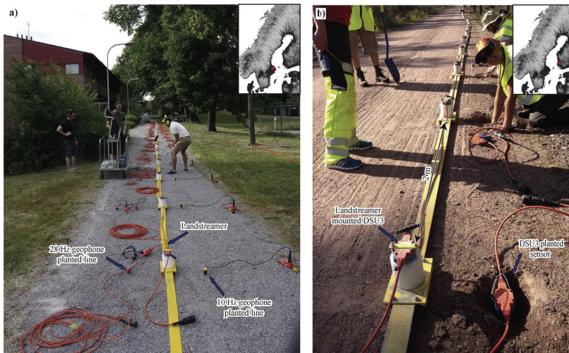
Figure 2. Photos showing details of the landstreamer versus planted geophones tested at the early stage of the development of the streamer. (a) Landstreamer was located in the middle of two planted geophone-type (10 Hz on the right-hand and 28 Hz on the left-hand side) lines. Note the difference in cabling involved for the planted lines and the streamer-mounted units. A sledgehammer was used as the seismic source in this study. (b) Side-by-side comparison between planted and streamer mounted 3C (DSU3, MEMS-based) sensors. This test was done to study different characteristics of the seismic wavefield registered on the streamer mounted sensors and if the sleds have some noticeable effects on the wavefield especially the horizontal components.
