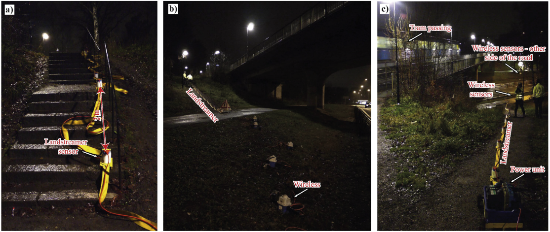
Fig. 7. Photos showing field condition along Line 2 at the access ramp of Stockholm Bypass at the Vinstå site. (a) Landstreamer units placed at the staircase as a part of the first spread deployment along this line, spacing of 4 m streamer segment reduced to 2 m. (b) Combination of the landstreamer sensors with 12 MEMS-based wireless recorders to cover the inaccessible zone; at the major road cutting the line into two segments. (c) Tram passing during the data acquisition, location of the wireless units on both sides of the road and a view showing the severe topographic variations from one side of the line to another.
