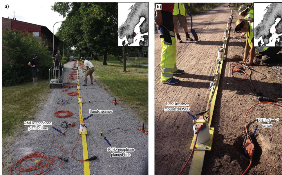
Fig. 2. Photos showing details of the landstreamer versus planted geophones test. (a) Landstreamer was located in the middle of two planted geophone-type (10 Hz on the right-hand and 28 Hz on the left-hand side) lines. Note the difference in cabling involved for the planted lines and the streamer-mounted units. A sledgehammer was used as the seismic source in this study. (b) Side-by-side comparison between planted and streamer mounted 3C (DSU3, MEMS-based) sensors. This test was done to study different characteristics of the seismic wavefield registered on the streamer mounted sensors and if the sleds have some noticeable effects on the wavefield especially the horizontal components. A Bob-cat drop hammer was used as the seismic source in this study.
