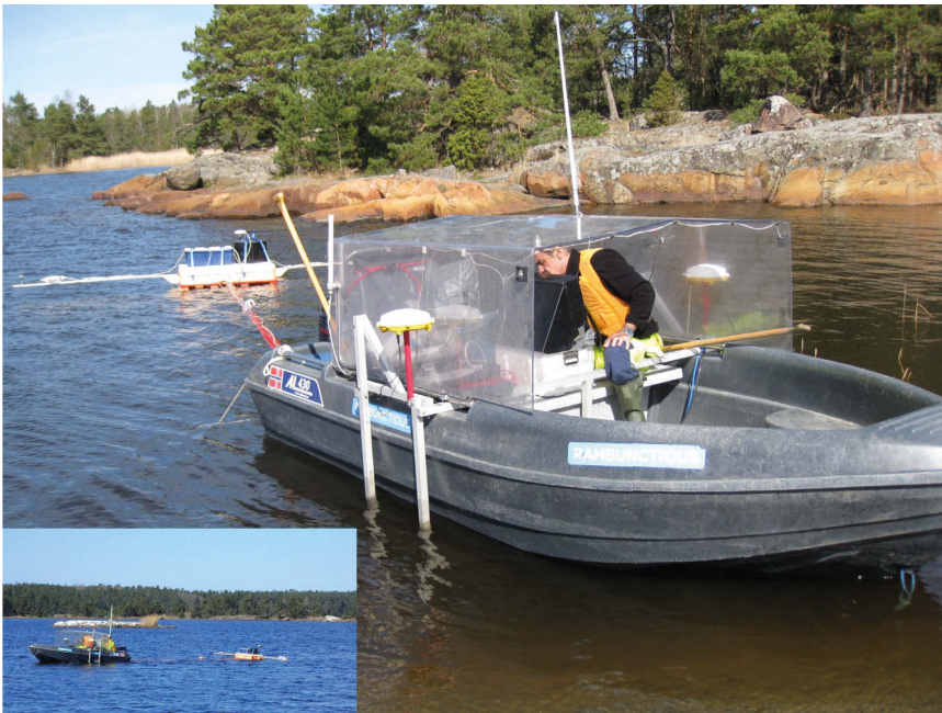
Figure 13. Photos showing the deployment of the boat-towed RMT system during the Äspö experiment.
