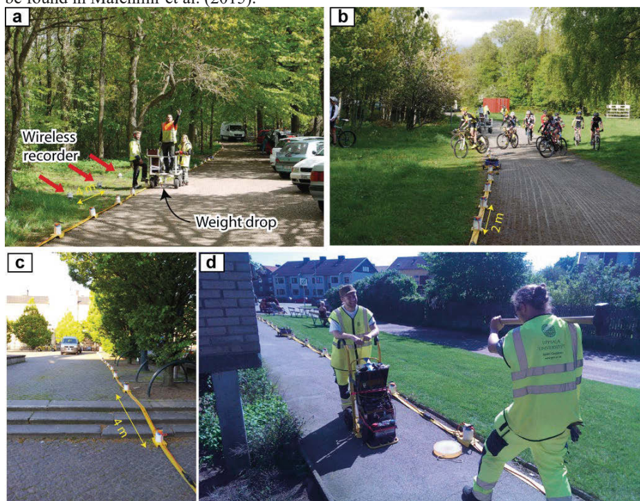
Figure 7. Field photos showing the acquisition conditions in the city of Varberg. (a) Combined seismic streamer and wireless recorders (often about 4 m apart) were used to acquire the data (along line 2 and parts of line 3; see Figure 1). (b and c) Ground conditions and (d) use of a sledgehammer for some of the lines in downtown Varberg. From Dehghannejad et al. (2017).
