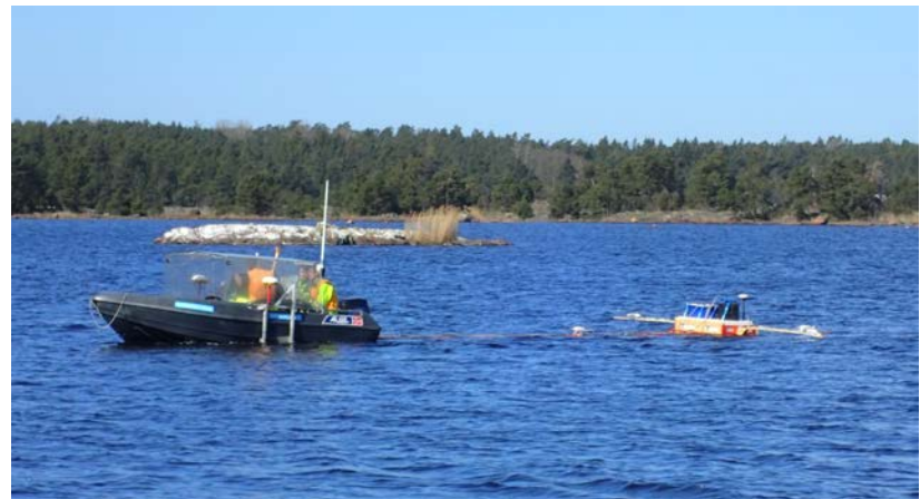
Boat-towed RMT system, Äspö
