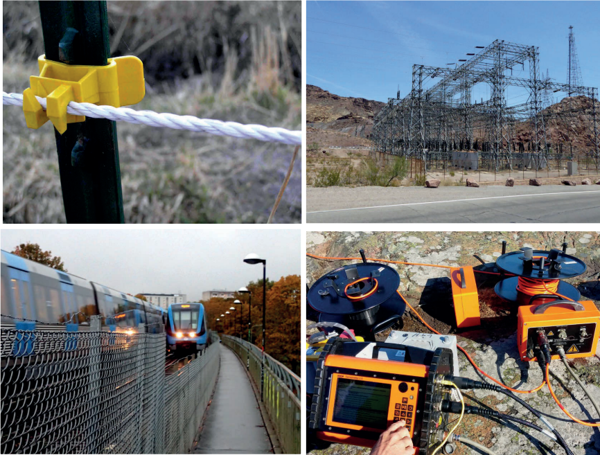
Figure 5. Different kinds of known sources that affect the measured potential and their typical signal characteristics: electrical fence - spikes (top left), power grid - harmonic noise (top right), tram running on DC - background drift (bottom left), DCIP instrument - square pulse train (bottom right).
