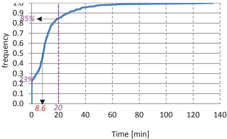
Figure 5.5 Cumulative function of actual grouting time for all 326 holes at the Bangård tunnel in the Stockholm City Line project (After Tsuji et al. 2012).
