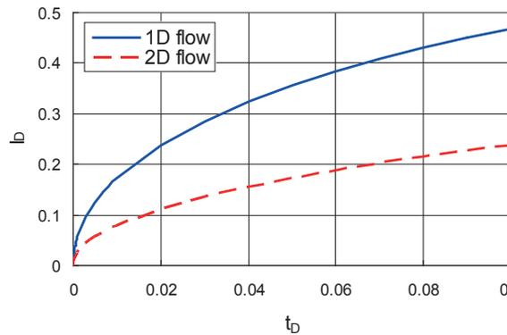
Figure 3.4 Relative penetration as a function of relative grouting time for different dimensionalities (Gustafson and Stille, 2005)
