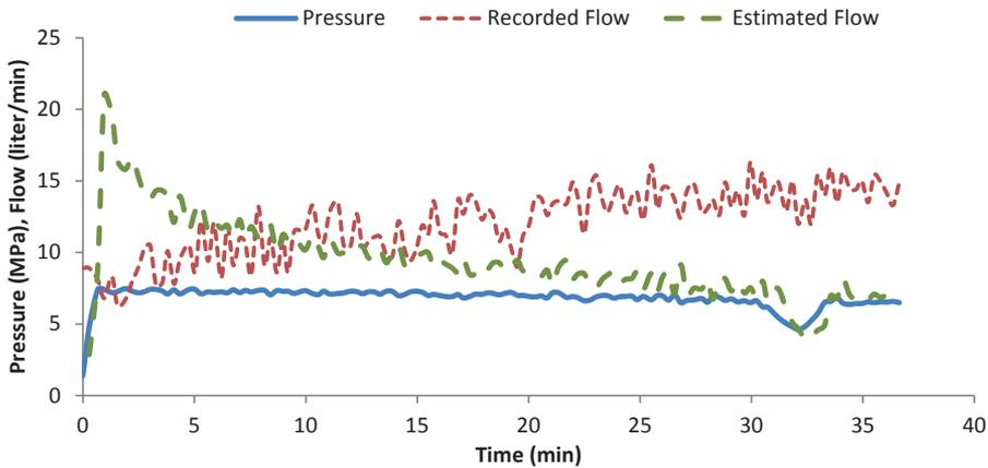
Figure 6.15 Estimated flow of grout in the fracture with average estimated aperture size of  $80\mu\text{m}$  during grouting.
