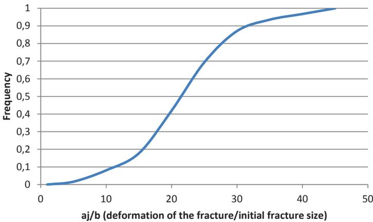
Figure 6.10 Cumulative function of the estimated increase in fracture aperture size in the zone with sand stone (62 holes). “ $a_j$ ” is the amount of deformation. “ $b$ ” is the initial fracture aperture size (as depicted in Figure 6.8.)
