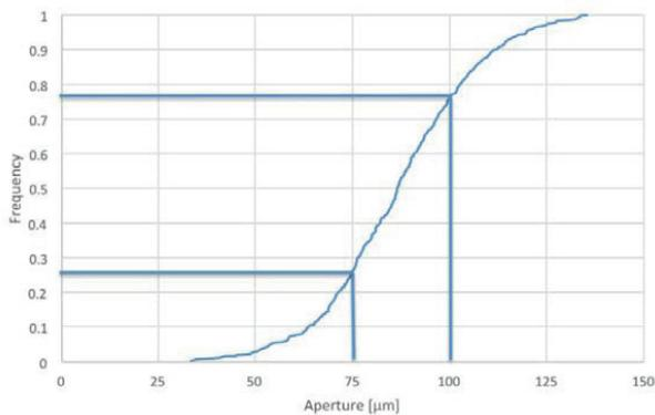
Figure 6.3 Cumulative function of the estimated aperture size by considering the flow of the grout inside the fracture using the RTGC (After Nikolaev, 2015). This Figure covers all of the fractures in the 3 regions depicted in Table 6.1.
