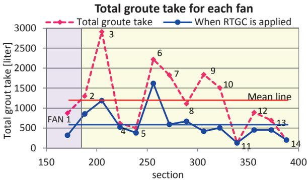
Figure 5.6 Comparison of the measured injected volume and the estimated grout volume based on the estimated penetration length. The aperture for each hole has been estimated based on recorded flow of grout (RTGC)
