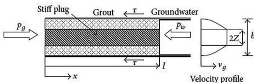
Figure 3.1 Grout penetrating a fracture (After Gustafson, et al., 2013)
