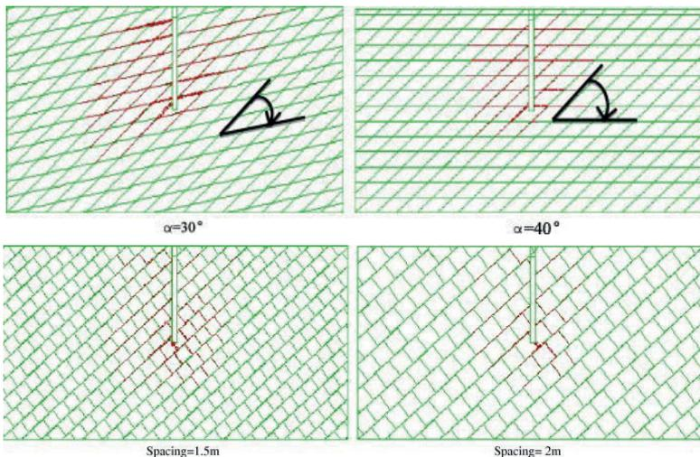
Figure 3.3 The effect of joint dipping on grout flow and grout penetration (red lines) around a borehole with different dipping (after Saedi, et al., 2013).
