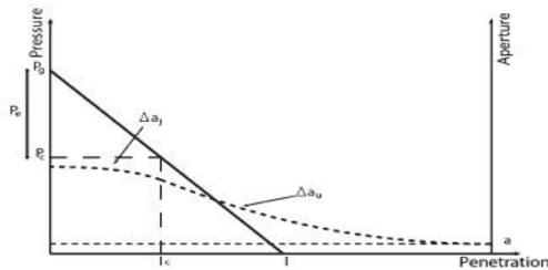
Figure 3.11 The principles of pressure and deformation. In this model the X-axis represents the radial distance from the bore hole. The pressure drops approximately linearly with distance and becomes zero at the grout front. The deformation is approximated by  $\Delta a_j$  in distance that pressure acts and beyond that is varied (After Gothäll and Stille 2009).
