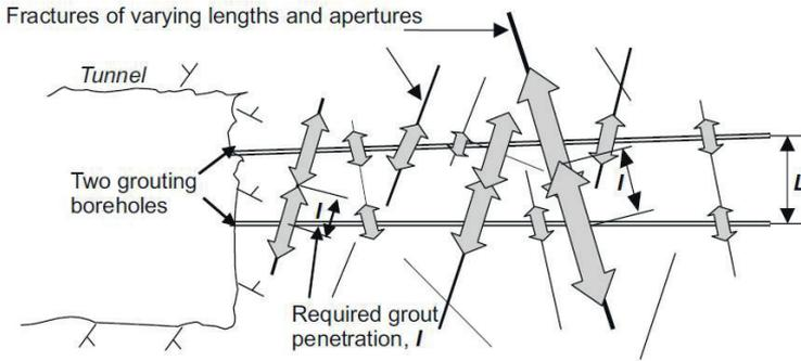
Figure 3.6 Illustration of the required minimum grout penetration.  $L$  is the distance between the grouting boreholes (after Funehag 2007).
