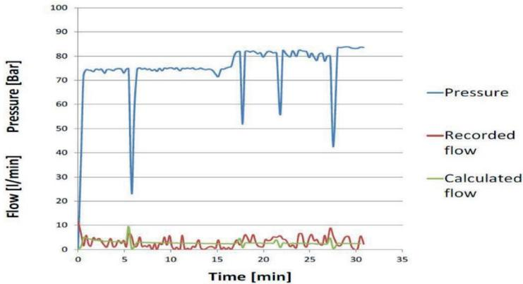
Figure 6.19 Example of a hole with limited grout take in fan 80472 (hole number 10) in the Holm-Nykirke project (After Nikolaev, 2015)
