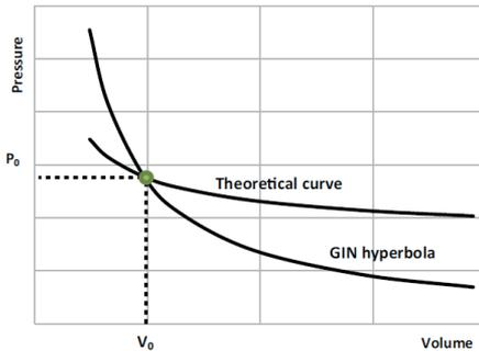
Figure 3.15 Grouting is completed at the intersection of the GIN hyperbola and the theoretical curve, where the injected volume of  $V_0$  confirms a sufficient spread of grout and the pressure of  $P_0$  limits the fracture deformation to the permitted level (after Rafi and Stille<sup>2</sup>, 2015).
