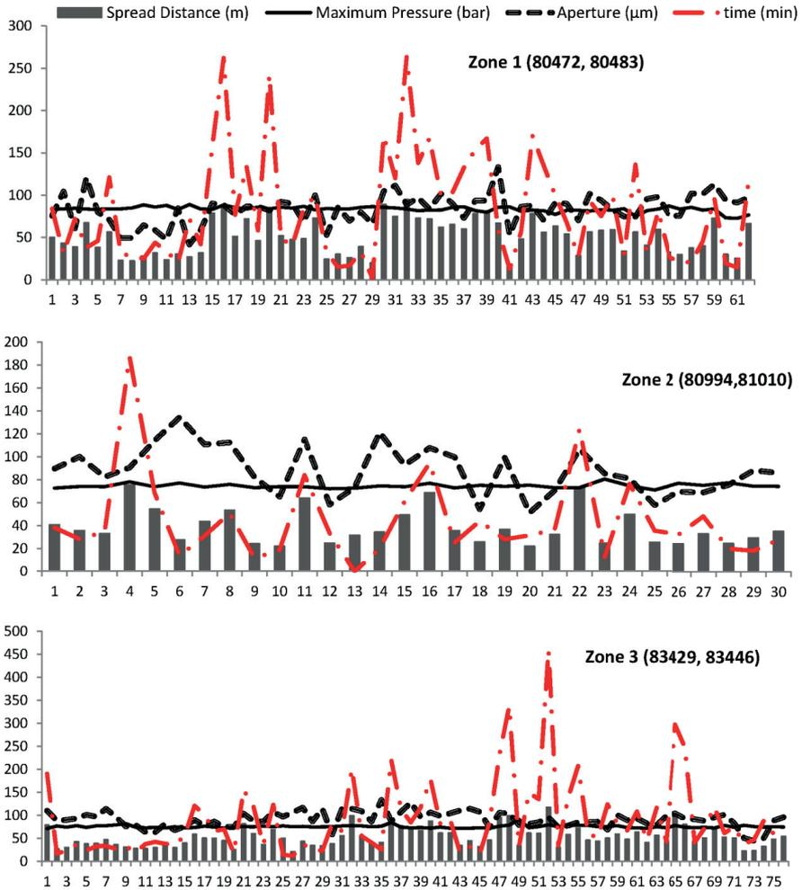
Figure 6.9 The effect of pressure, time and aperture size on the distance of the grout spread (5 fans) in the Holm-Nykirke project.
