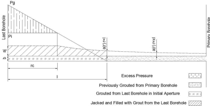
Figure 3.13 Mechanism of elastic jacking. Fracture deformation is extended outside the grouted zone, which may open the previously grouted section from primary borehole (after Rafi and Stille<sup>1</sup>, 2015).
