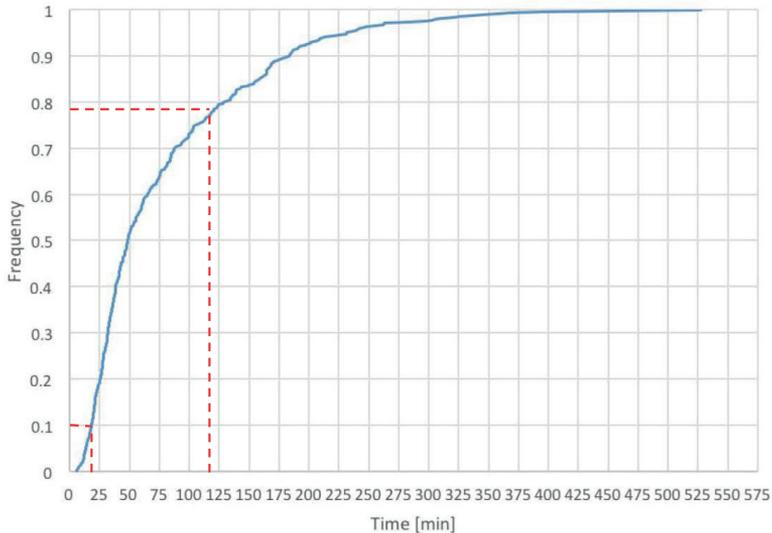
Figure 6.6 Cumulative recorded grouting time in each hole in the Holm-Nykirke project (After Nikolaev, 2015). Around 10% of the grouting work was finalized in less than 20 minutes and around 80% of the holes have been grouted in less than 2 hours.
