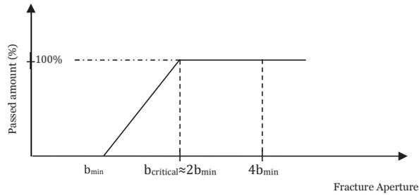
Figure 3.12 Increasing the aperture size beyond the size of the critical aperture will not improve penetrability (after Rafi and Stille<sup>1</sup>, 2015).
