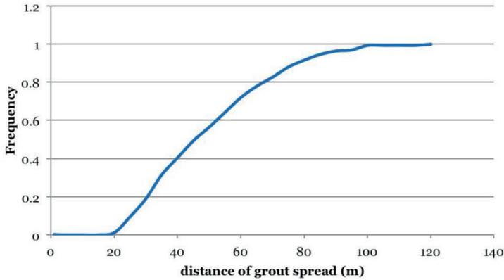
Figure 6.7 Cumulative function of the distance of the grout spread in the sandstone zone
