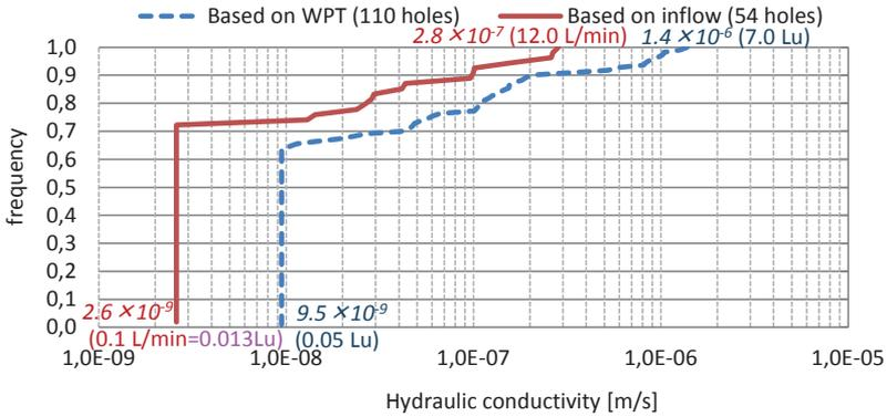
Figure 5.2 Cumulative function of transmissivity in each hole based on water pressure test results compared with that based on inflow measurements (after Tsuji, et al. 2012).
