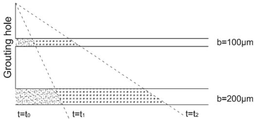
Figure 3.14 When several fractures are grouted, the same percentage of maximum penetration length is traversed at each time interval for all the fractures, regardless of the aperture size (after Rafi and Stille<sup>2</sup>, 2015)
