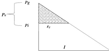
Figure 3.10 Excess pressure ( $P_e$ ) is due to the difference between grouting pressure and critical pressure (dotted zone) (after Rafi and Stille, 2014).
