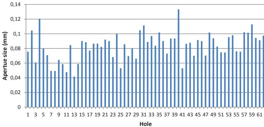
Figure 6.8 The size of the hydraulic apertures in the sandstone zone
