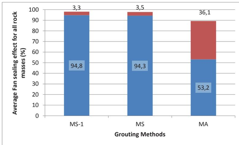
*Figure 1.1 Total average fan sealing effect after grouting and re-grouting (after Dalmalm 2004)*
