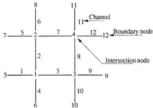
Figure 3.2 Defining a network of fractures as boundary node, intersection node and channel for establishing the matrix (after Hässler, 1991)
