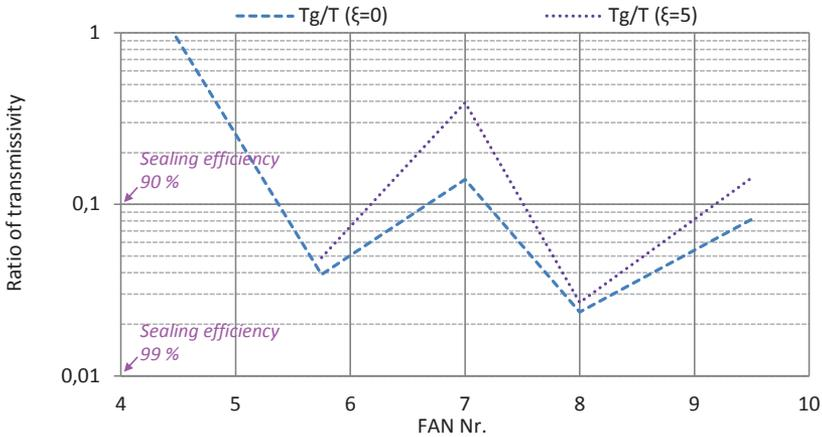
Figure 5.7 Reduction of transmissivity by grouting at the Bangård access tunnel in the Stockholm City Line project (After Tsuji et al. 2012).
