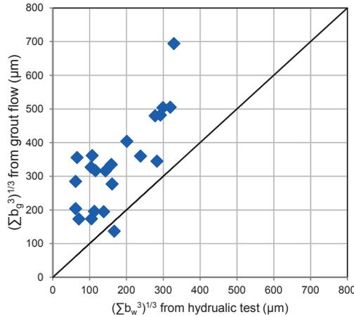
Figure 3.5 Comparison of fracture aperture size obtained from the Lugeon test and the Real Time Grouting Control method, which consider filling the voids with Bingham material using data from the Stockholm City Line project. It is illustrated that the latter measurement method estimates a larger fracture aperture size (After Tsuji, et al., 2012).
