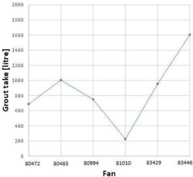
Figure 6.4 The estimated injected volume corresponding to 10 meter of radial grout spread in different fans (after Nikolaev, 2015)
