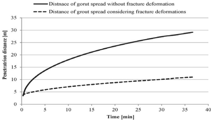
Figure 6.18 Comparison of the distance of grout spread with an initial aperture of  $62\mu\text{m}$  (30m) and the deformed fracture that opens up to 2 mm, (11 m). This means that the ratio of  $l/l_c$  is around 2.7.
