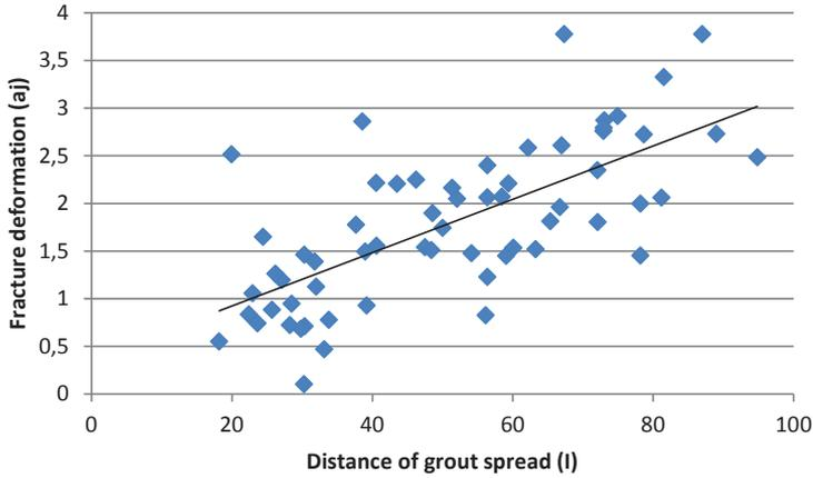
Figure 6.11 Correlation between the distances of grout spread with fracture deformation. Deformation is in millimetre and distance of grout spread is in meter.
