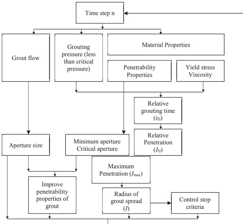
Figure 3.8 Online application of the Real Time Grouting Control Method
