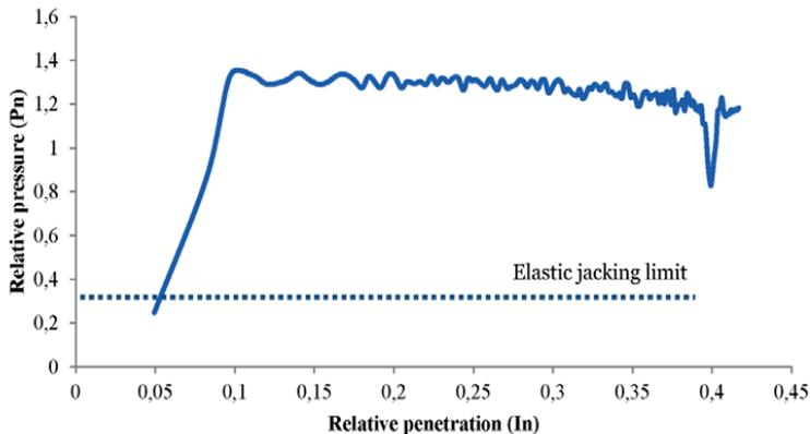
Figure 6.17  $P_n$ - $ln$  compared with the elastic and ultimate jacking limits in hole 10 of fan 80472. The grout spread up to 30 meters from the boreholes
