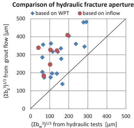
Figure 5.3 Comparison between the hydraulic fracture apertures based on hydraulic test  $(\Sigma b_w^3)^{1/3}$  and that based on the grout flow  $(\Sigma b_g^3)^{1/3}$  for 27 boreholes (after Tsuji, et al., 2012)
