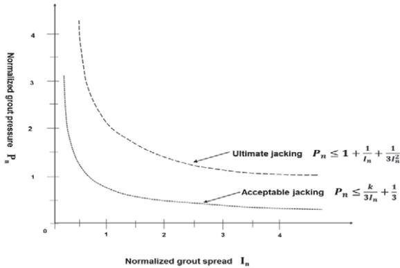
Figure 3.9 Maximum normalized pressure as a function of normalized grout spread for both the ultimate limit state (Eq.3.7) and the acceptable limit state (Eq.3.8). The curves are calculated for  $P_w = 0$  (after Stille, et al., 2012).
