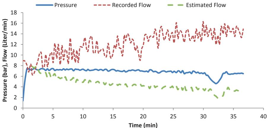
Figure 6.16 Estimated flow of grouting considering the initial estimated aperture size of  $62\mu\text{m}$ .
