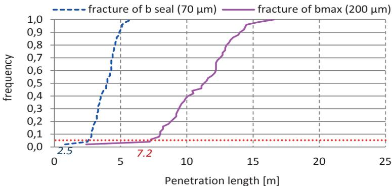
Figure 5.4 Cumulative function of grout spread for 50 holes with 2D grout flow at the Bangård tunnel in the Stockholm City line project (After Tsuji et al. 2012). The distance of grout spread has been estimated in smallest fracture to be sealed ( $70\mu\text{m}$ ) and largest existing fracture ( $200\mu\text{m}$ ).
