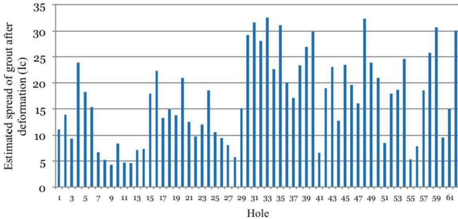
Figure 6.13 Distance of grout spread in deformed fracture of “aj+b” (lc) in the zone with sandstone.
