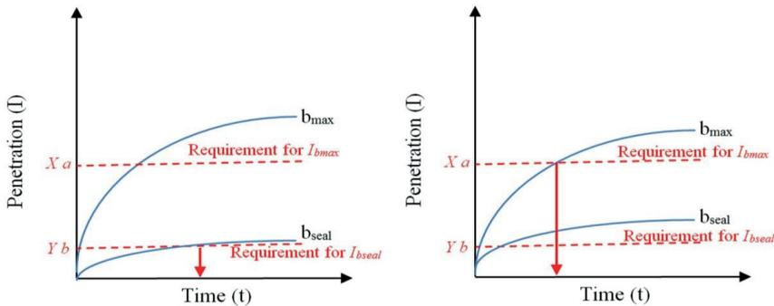
Figure 3.7 Illustration of the basic stop criteria. To the left, grouting is stopped when the distance of grout spread in the finest fracture to be sealed ( $I_{bseal}$ ) exceeds the design requirements. To the right, grouting is stopped when the grout spread is equal to the maximum allowed (Tsuji, et al., 2012).
