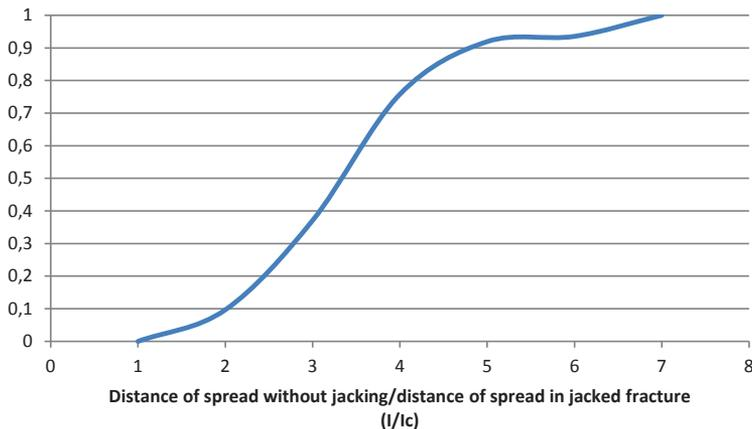
Figure 6.12 Cumulative function of the ratio of distance of grout spread in initial fracture of “b” (l) to the deformed fracture of “aj+b” (lc) in sand stone zone.
