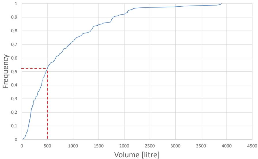
*Figure 6.5 Cumulative measured injected grout volume in different boreholes (after Nikolaev, 2015)*
