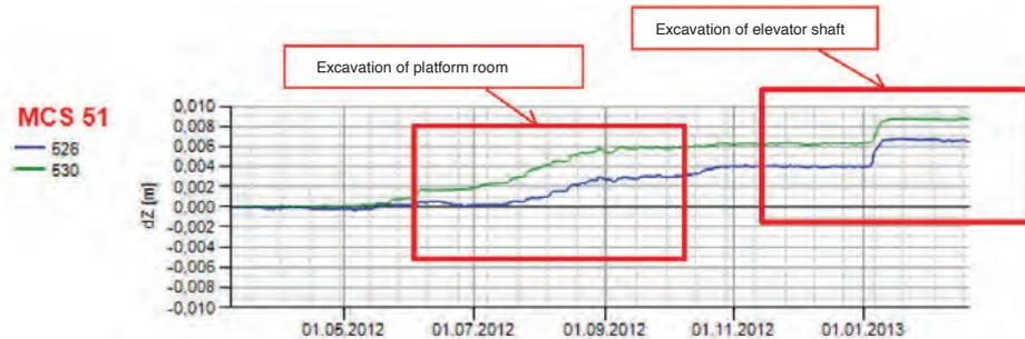
Figure 11 Results from measurements with liquid levelling gauges LLS 526 and LLS530 (From Johansson et al. 2013).
