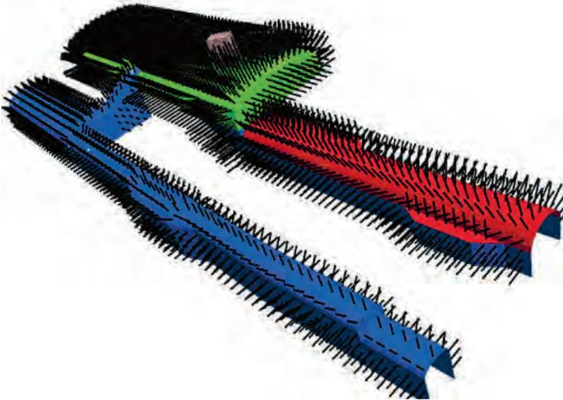
Figure 32 Excavation of last part of the tunnel U2 and installation of support.
