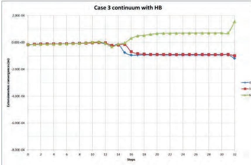
Figure 64 Simulated extensometer response in meters vs. simulation step for stress case 3, continuum elasto-plastic (modified H-B).
