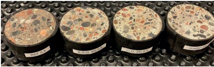
FIGURE 3.2. Four sawn concrete cylinders ( \varnothing = 100 mm height = 85 mm). Neoprene layer applied to all surface except the top.
