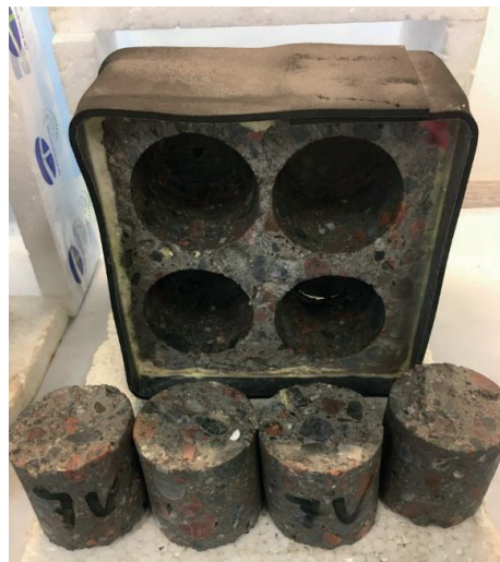
FIGURE A4.5. Example of cored specimens from a concrete slab exposed to F-T testing conditions.
