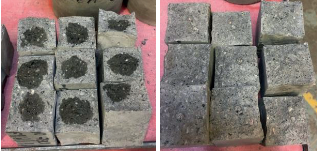
FIGURE 1.6. Plan view of cement mortar prisms 40 mm x 40 mm post destructive testing, w/c = 0.50 at 28 days
