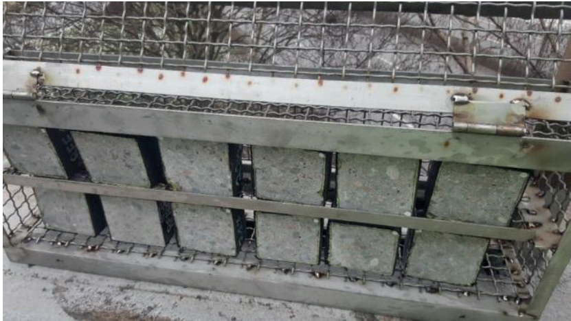
FIGURE A6.1. January 2018 original batch in place; REF x2 plus TAG x2 (O.O. & R.S.O) and “silane” based x2. All hydrophobic concretes dosed at 3% (based on cement weight). w/c = 0.40.
