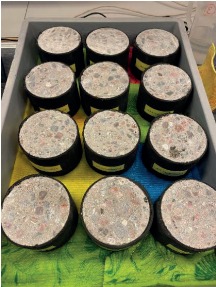
FIGURE 3.1. Water absorption test of \text{\O}100 mm & 80 mm thick concrete specimens; w/c = 0.50. Three specimens per recipe. Specimens placed on a textile-based material which itself lies on a plastic raised bed filled with water. Sawn concrete exposed to water (bottom) and the ambient air (top). A 3 mm thick neoprene layer was applied to the sides of the cylinders.
