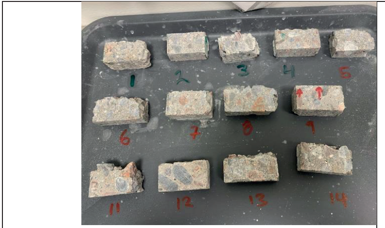
FIGURE A 2. Side profile of the top surfaces (in contact with freezing medium) of the concretes prior to thin section preparation. HXL or nr. 10 was not able to be prepared with a diamond saw and was not included in the thin section analysis. 1 = REF 0,40 w/o AE , 2 = REF = 0,40 + AE, 3 =REF 0,40 w/o AE (crushed agg), 4= O.O. 3% + AE (5.4%), 5= O.O. 3% w/o AE, 6= R.S.O. w/o AE, 7= R.S.O. + AE (6.3%), 8= H.X.L. 1% w/o AE, 9= HMP 1% w/o AE, 11 C.H.A. 1 3% w/o AE, 12 C.H.A. 2 3% +AE , 13 = C.H.A. 2 2.1kg/m3 w/o AE, 14= C.H.A. 2 3% (0.40) w/o AE.
