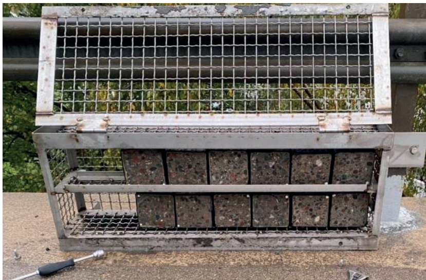
FIGURE A6.3. October 2020 original testing samples, very clean around the specimen cage.
