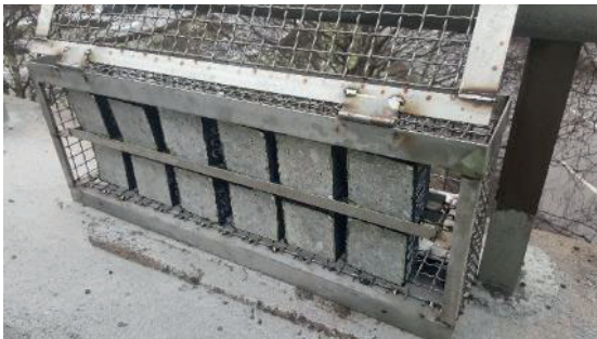
FIGURE 3.6. The initial field station installed 11th January 2018. The concretes are 100 mm sided with neoprene outer shell, exposing only the sawn surface. Concrete age at time of exposure ca 3 months.
