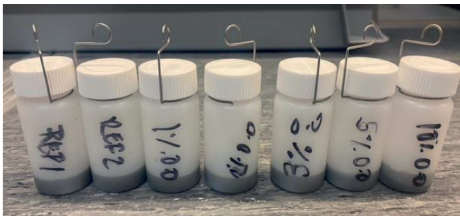
FIGURE 3.5. Plastic ampoules used for iso thermal calorimetry, ca 7.00 g sample per ampoule.
