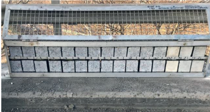
FIGURE A6.2 April 2019 installation of the longer cage with 12 recipes for this study (13-15 are from another project).
