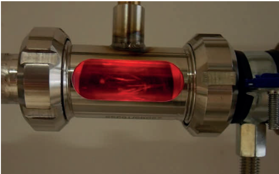
Figur 4. Synglas med passerande kavitationsbubblor i laserridå. Sight-glass with cavitation bubbles passing the laser-curtain.
