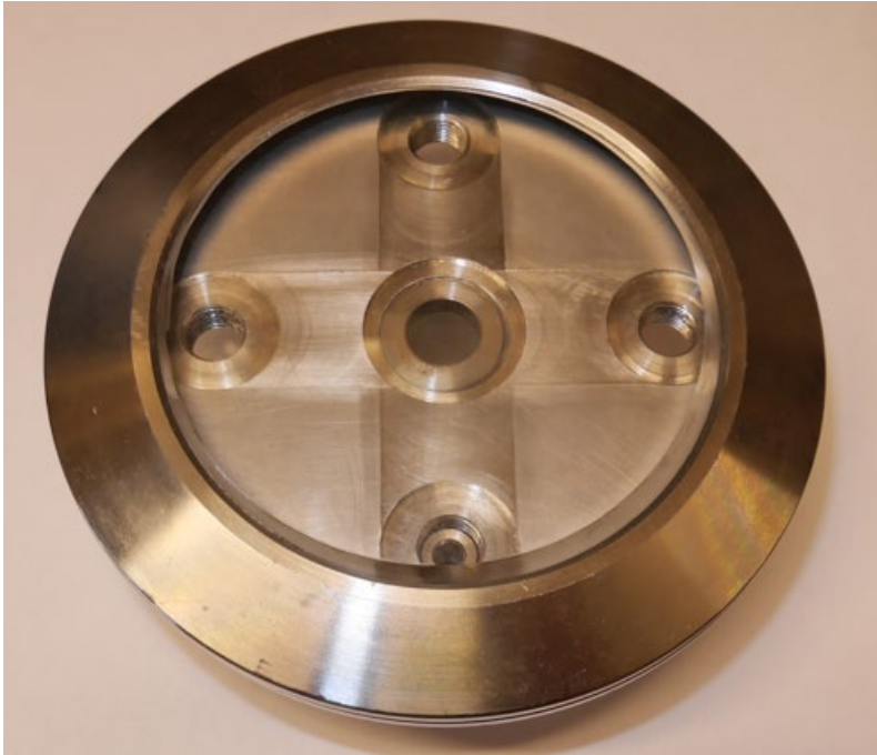
Figur 20. En mindre version av kort spalt tillverkad vid LTH. Ytterdiameter 120 mm. A smaller version of the "kort spalt" concept manufactured at LTH. The outer diameter is 120 mm.
