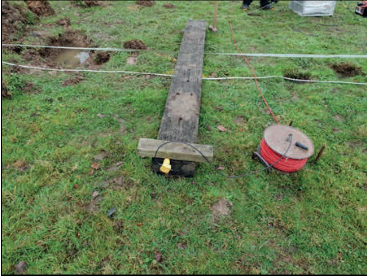
Figure 3 Wooden beam as SH source for the London test
