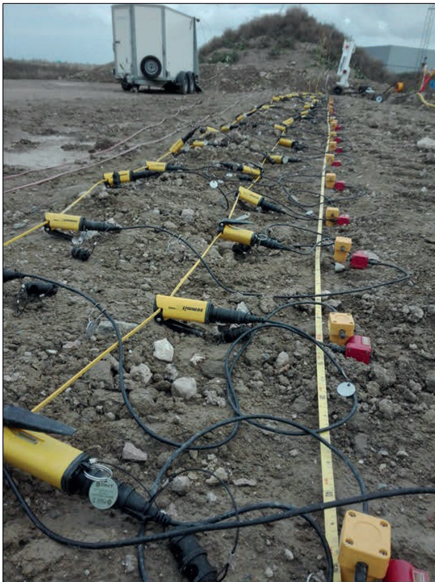
Figure 11 Example of geophones layout: Layout 3 with 0.5 m spacing, 4.5 Hz geophones. Yellow receivers are the vertical component geophones, while the red ones are the horizontal (in-line) component geophones.
