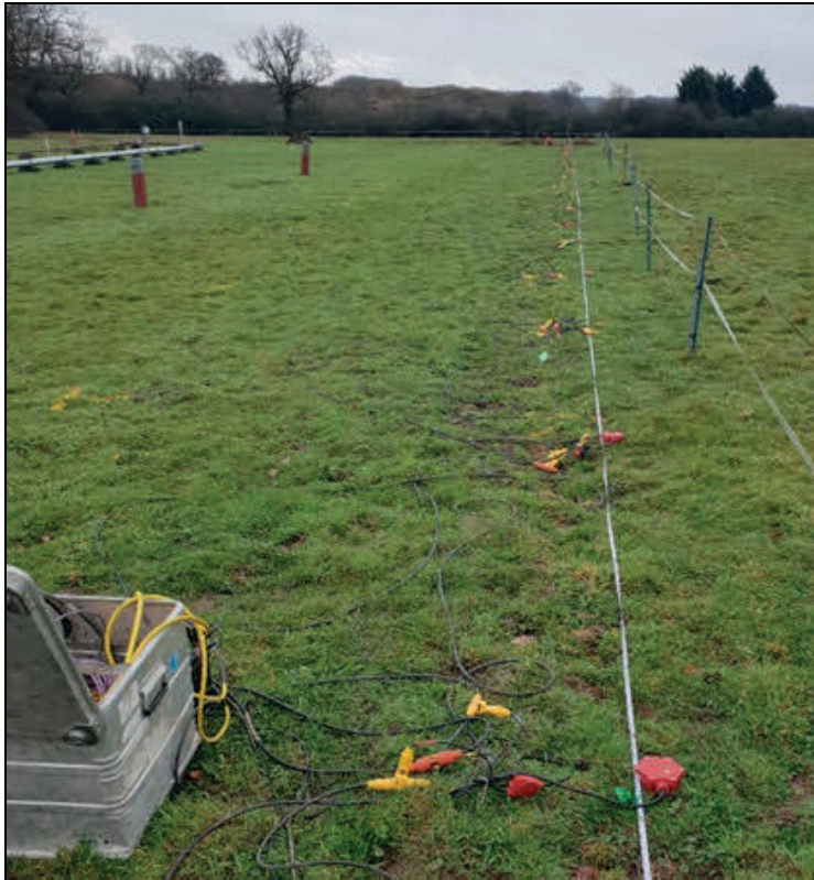
Figure 2 Line of 3-axial geophones for the London test
