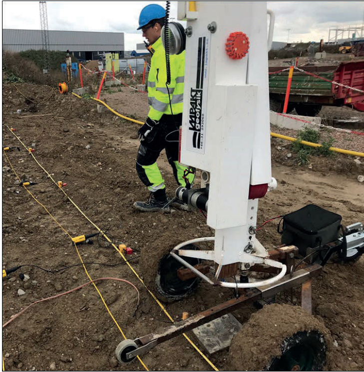
Figure 4 ESS100Turbo accelerated weight drop. The Summit X One Remote Units are also visible together with two geophones next to the wheel of the weight drop.
