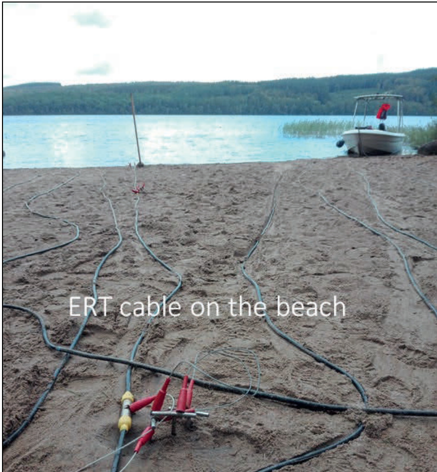
Figure 15 ERT cable and one installed electrode on the beach. In the water there are no extra connectors or electrodes except the one moulded into the cable.
