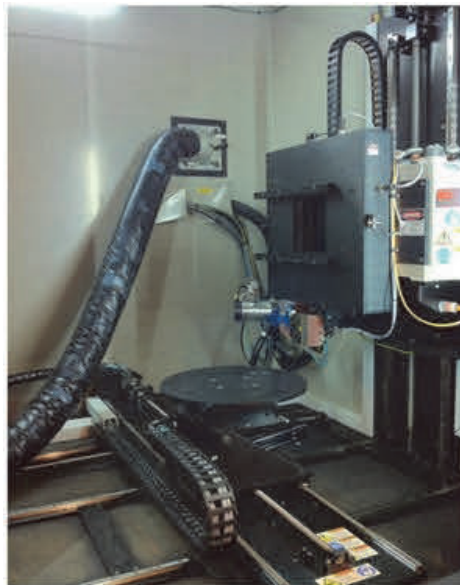
Figur 6. Röntgenstrålkällor i NSI X5000 systemet. (Foto: KTH Bygghälsa). Figure 6. X-ray sources in NSI X5000 system (Photo KTH Civil and Architectural Engineering).
