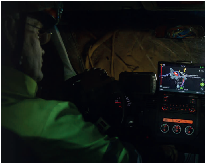
Figure 7. Navigation underground where every vehicle and position of equipment is visible in the mine (Mobilaris, 2020).
