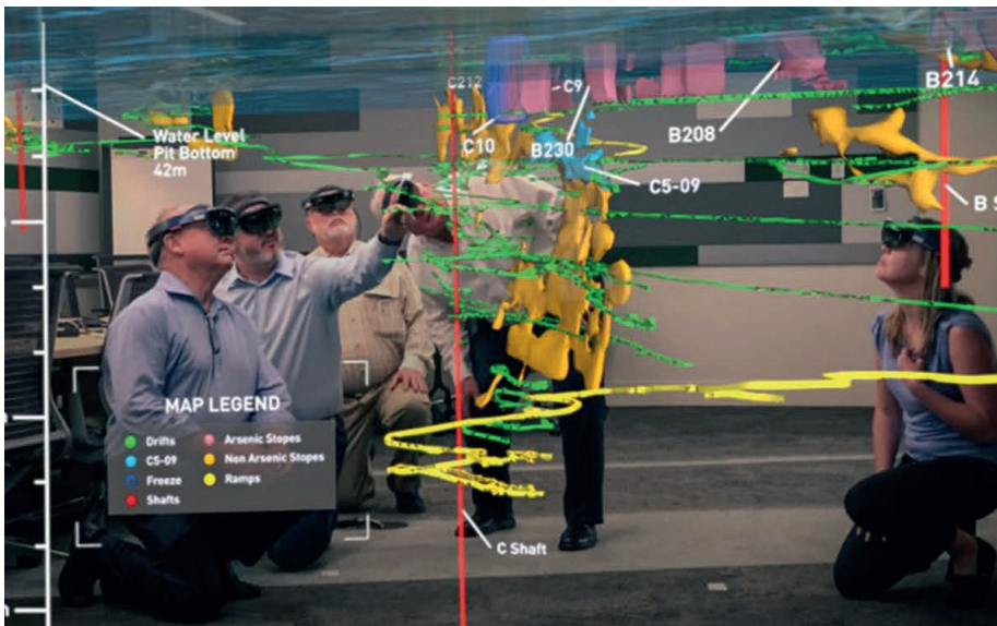
Figure 6. 3D-models of the Giant mine used as communication and discussion tool (CIM News Magazine, 2018).
