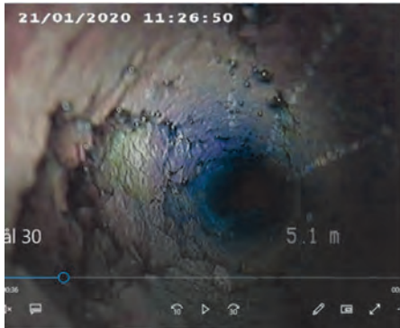
Figur 2. Hål nr 30, sprickor. Figure 2. Hole no 30, cracks.
