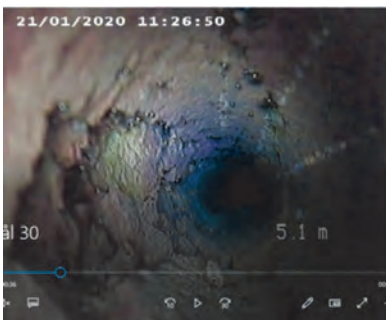
Figur 10.8. Hål nr.30, sprickor. Figure 10.8. Hole No.30, cracks.
