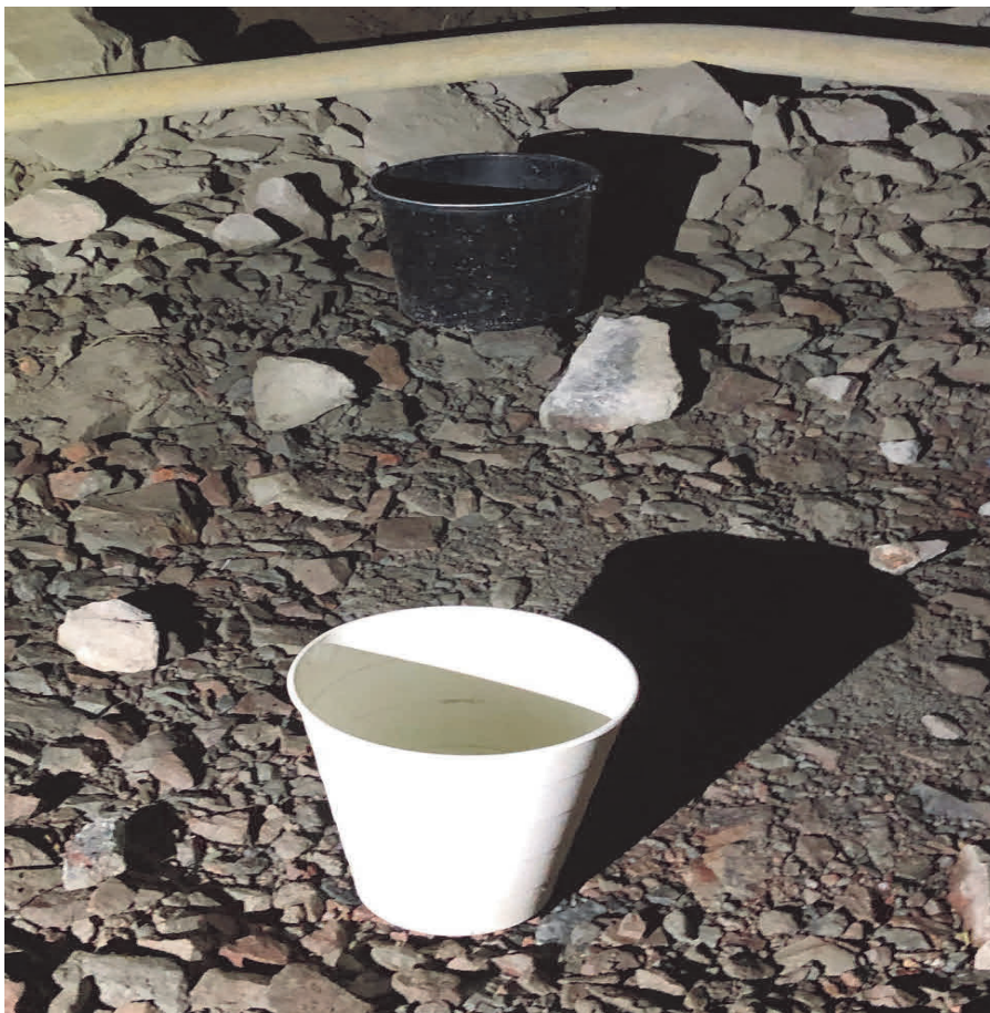
Figur 10.15. Droppkartering. Figure 10.15. Drop mapping.
