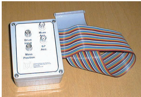
Figur 7. IVI adapter med koppling till ingångssignal, motviktsacceleration, motviktsposition samt markplattans acceleration, den signal som är närmast det man sänder ut i marken. Adapter from IVI with BNC:s for sending an input signal and measuring the mass acceleration, the mass position and the baseplate acceleration, the signal closest describing what is transmitted into the ground.
