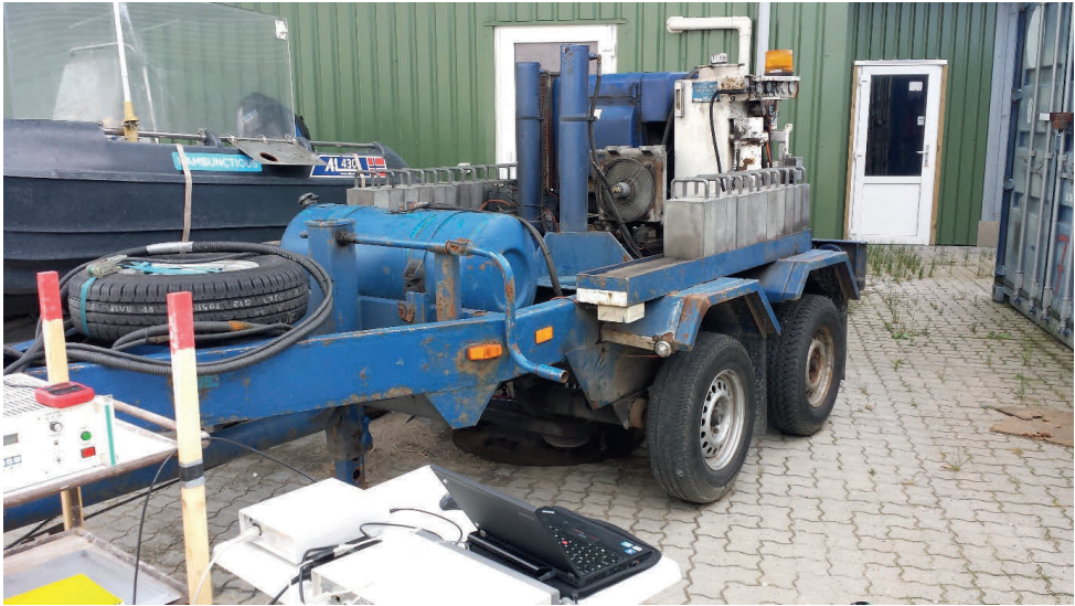
Figur 12. I denna bild visas tydligt vibratorns bottenplatta (Base Plate). Hela ekipaget hissas upp och vilar på denna platta. Plattans acceleration är vår mätsignal och den hämtas via IVI-adaptern och BNC-kontakten Base Plate Acceleration – BP Acc. In this picture the baseplate of the vibrator is demonstrated. The entire vehicle is elevated and everything rests on this plate when operated. The acceleration of the plate is our measurement signal and it is retrieved from the IVI-adapter and the BNC "Base Plate Acceleration" - BP Acc.
