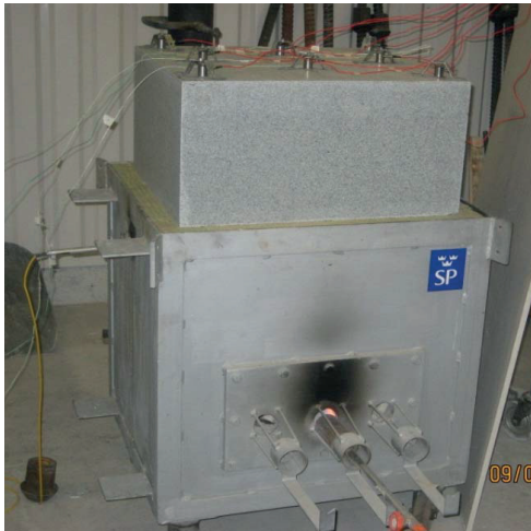
Figure 21 Rock block (granite) placed on the furnace.
