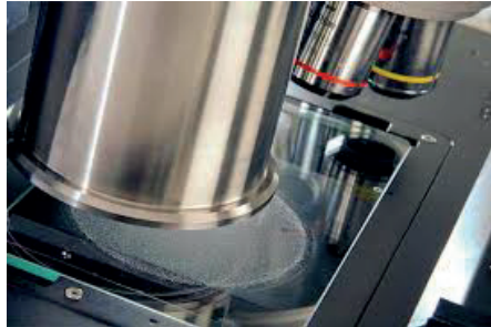
Figure 7: Measurement with a Malvern Morphologi G3
