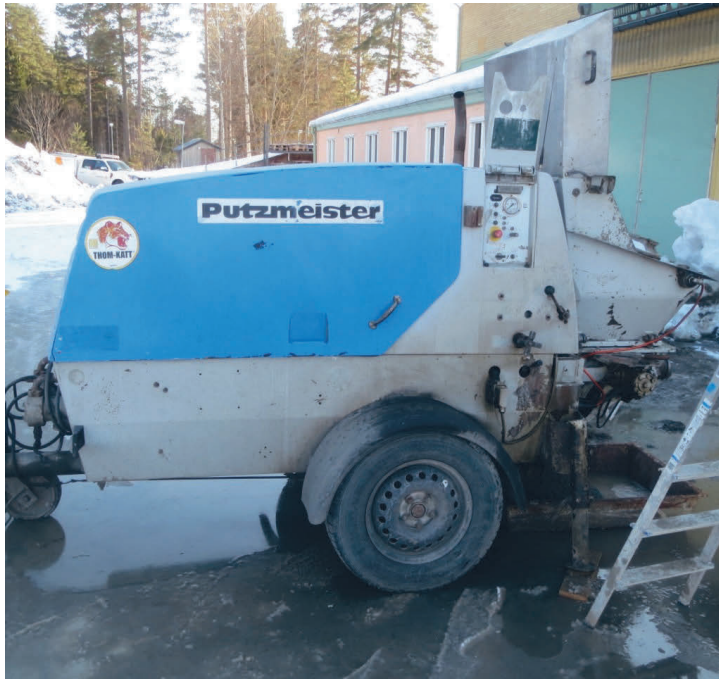
Figure 2.3 Concrete pumping machine, Putzmeister, THOM-KATT (TK 25). Sprutbetongpump, Putzmeister, THOM-KATT (TK 25).
