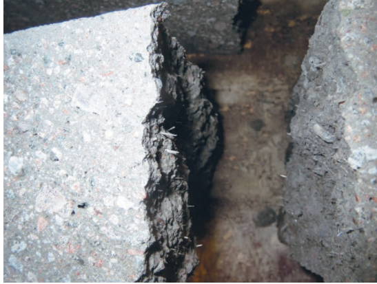
Figure 3.4. Glass fibre in failure surface of beam tested in bending. Glasfiberbrott i böjprovad balk.
