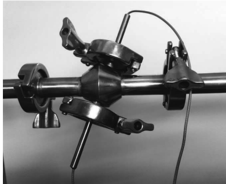
Figure 4 Flow adapter cell consisting of delay line ultrasound transducers
