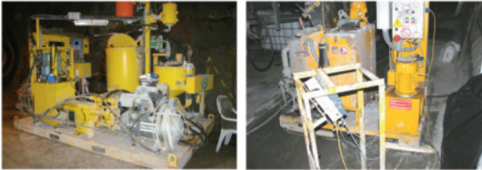
Figure 3-3. Example of grouting rigs. The photograph to the left is from the research facility at Äspö. The photograph to the right is from a project in the Telia tunnels.
