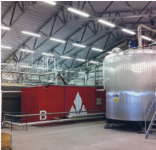
Figur 4. Tillverkarstation för emulsion. Mixing plant for pump emulsion (Foto Forcit)
