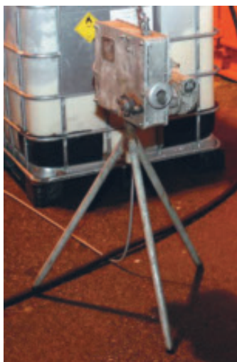
Figur 14. Bärbar slangmatare. Portable hose feeder (Foto EDZ-Consulting)
