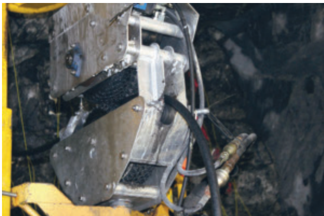
Figur 11. Slangmatare. Hose feeder (Foto EDZ-Consulting)
