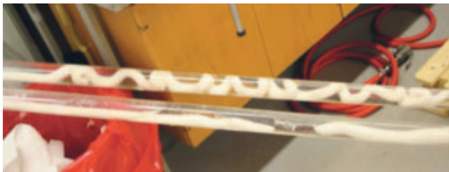
Figur 20. Avbrott i laddsträng. Disruption of an emulsion string (Foto EDZ-Consulting)
