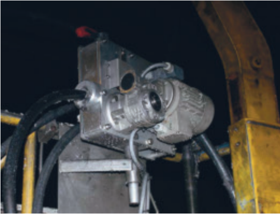
Figur 12. Slangmatare. Hose feeder (Foto EDZ-Consulting)
