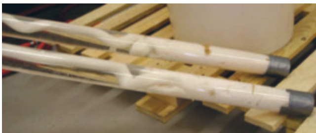
Figur 21. Bottenladdning. Bottom charge with pump-emulsion (Foto EDZ-Consulting)
